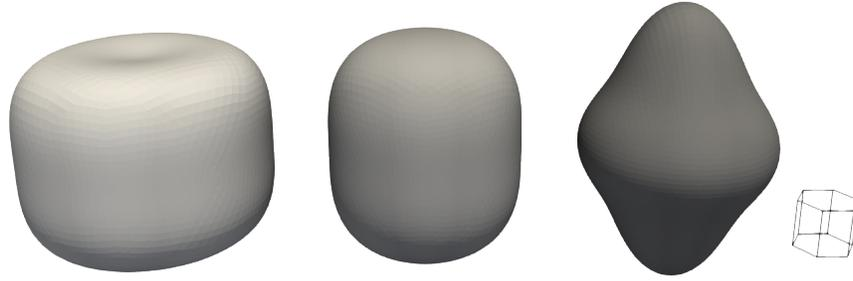
Figure 2.4 Directional stiffness in lattice frame coordinates illustrating each of the three representative instances of HCP elastic anisotropy listed in Table 2.2; from left to right and light to dark: “marshmallow”, “capsule”, and “spin”.
