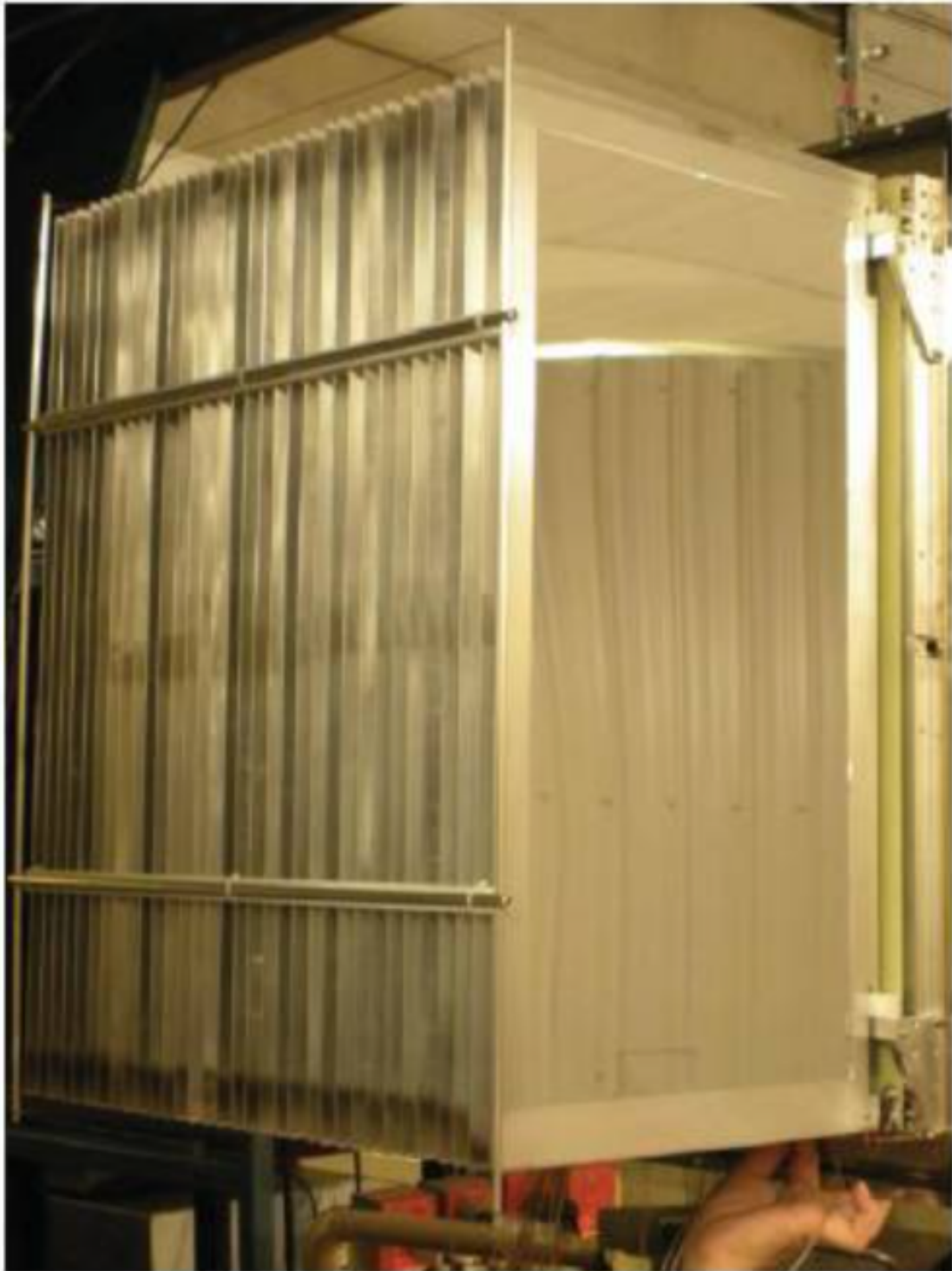
Figure 2.8 Unhoused view of the ion chamber at the focal plane of the S800. 16 parallel-plate ion chambers are stacked perpendicular to the beam axis (left to right) and cover an active area of \approx 30 \times 60 cm. When housed, the chamber contains a mixture of 90% argon 10% methane, typically at a pressure of 300 torr. The picture has been adopted from Ref. [21].
