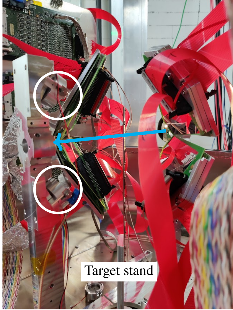
Figure 3.1 FABLE arranged in the front-back configuration for recording breakup fragments in coincidence with large angular separation at both forwards and backwards angles. The beam axis and direction is indicated with the cyan arrow. The target is placed at a 45^\circ angle with respect to the beam. Silicon beam monitors were mounted at forward angles, indicated by the white circles, to measure elastic scattering for normalization. In this configuration, the breakup and incomplete fusion yields from ^7\text{Be} on ^{208}\text{Pb} were measured.
