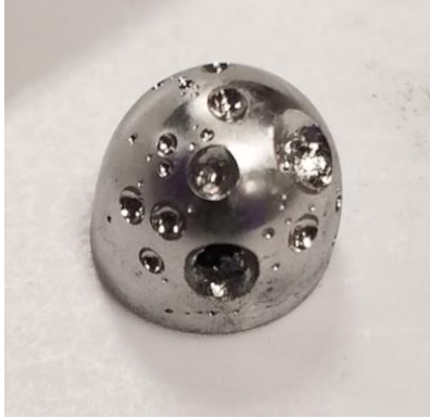
Figure 3.2: The bottom view of an extracted ingot of a Germanium-rich sample.
