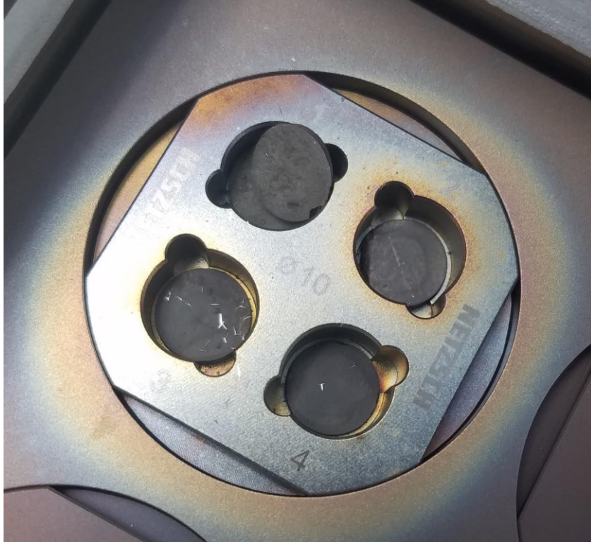
Figure 3.7: An image of four LFA samples in the 4-sample carousel inside the LFA.
