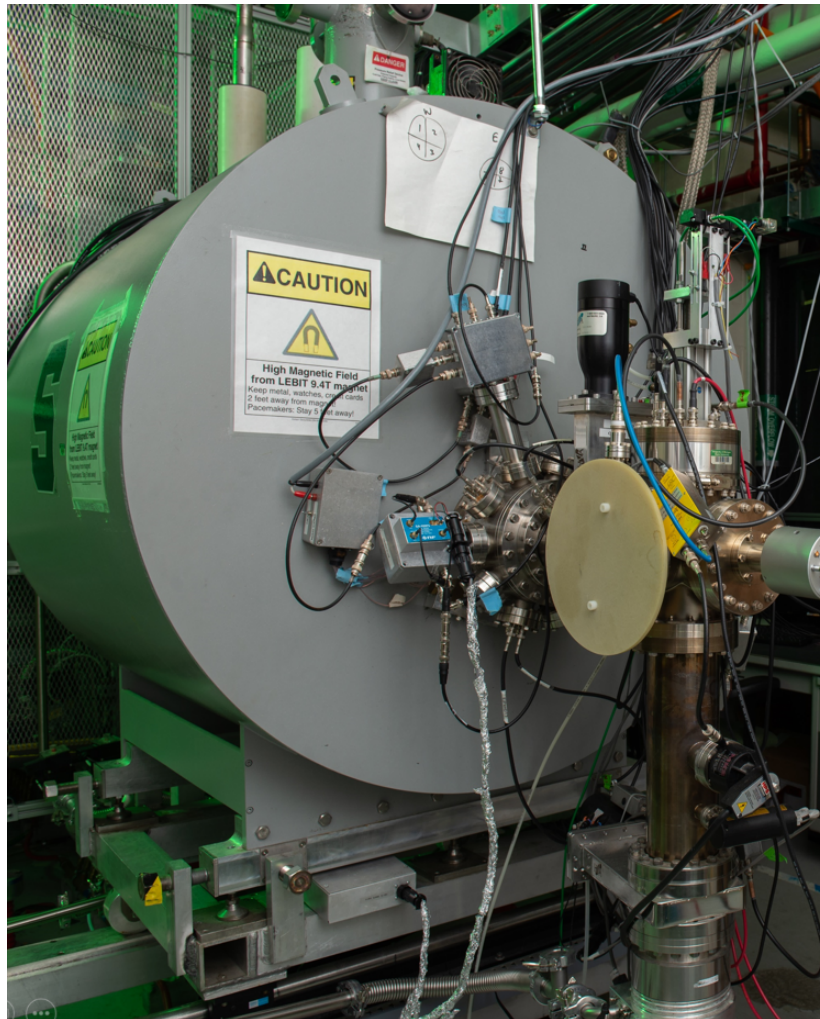
Figure 3.3 Image of the 9.4 T Penning trap mass spectrometer at the Low Energy Beam Ion Trap (LEBIT) facility.
