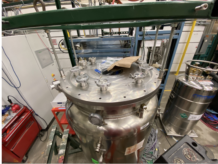
Figure 5.2 Test fitting of the top flange to the testing Dewar. Flange was mated to the Dewar and then pumped down to vacuum level and leak checked.
