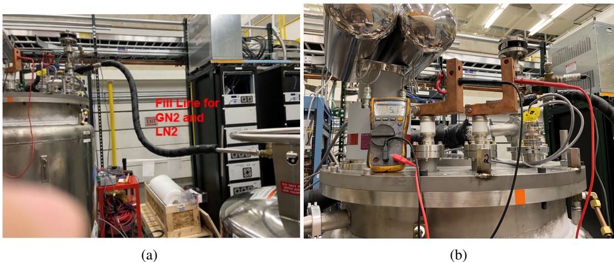
Figure 5.20 a) Picture of liquid nitrogen filling process for pre-cooling of coil. b) Resistance monitoring of the coil for internal temperature verification.
