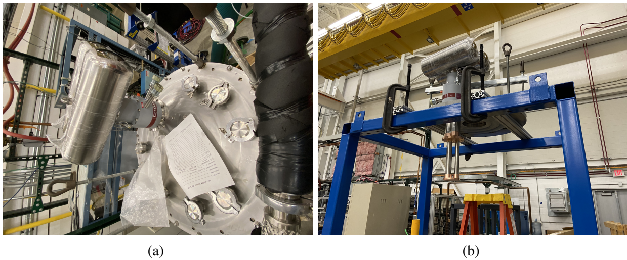
Figure 5.3 a) Cryocooler test fitted to the testing top flange while mounted in the Dewar. b) View of the cryocooler cold head positions while mated to the top flange.
