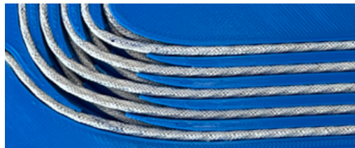
Figure 4.4 New location of the turn to turn transition area demonstrated on a sub-scaled flat prototype winding [20].
