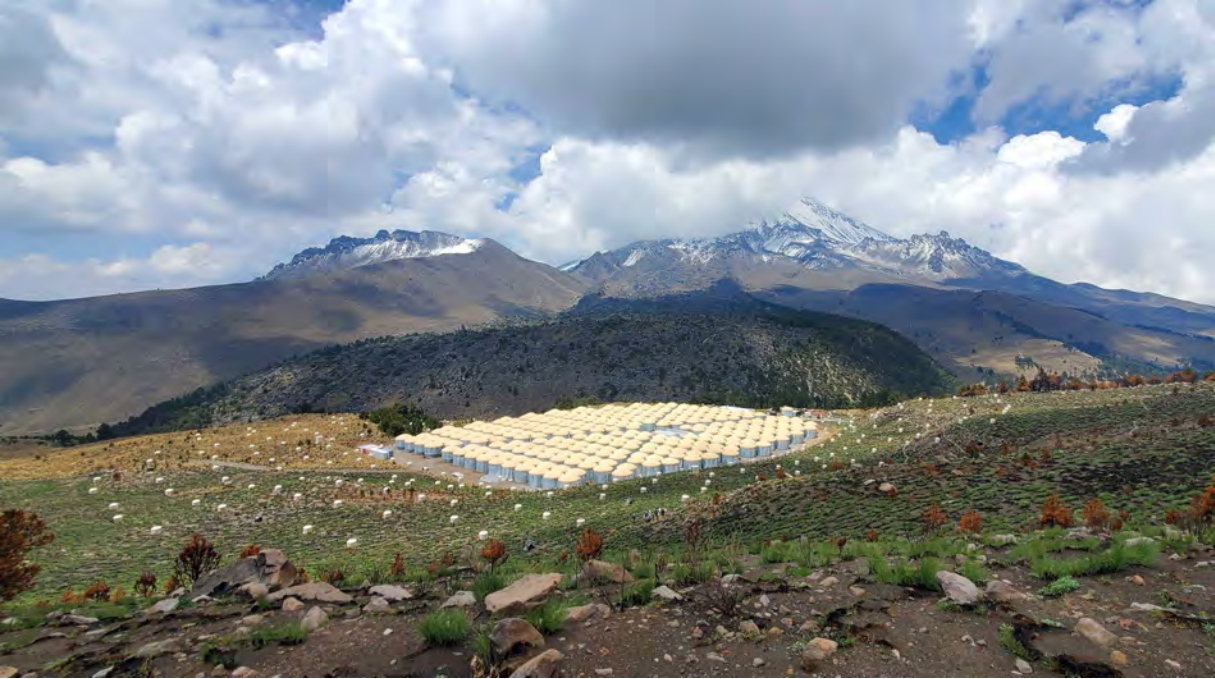
Figure 2.1 Photo of the HAWC detector that I took on May 17, 2023. Main array is centered in the photo and comprised of the larger tanks. Outriggers are the smaller tanks around the main array.
