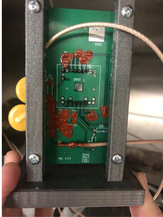
Figure 5.3: PMT base PCB used for the initial characterization of each PMT. PCB is fastened to calibration stand support structure and its components are painted with insulating varnish to prevent discharges.
