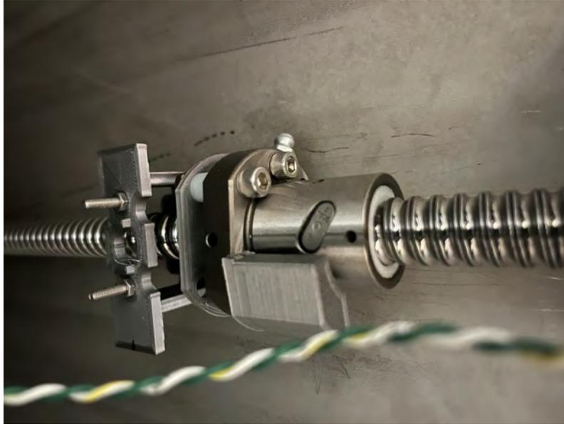
Figure 5.7: Up close view of LED holder assembly. It fastens to the nut of the ball screw and top of the slider block to group the separate components together.
