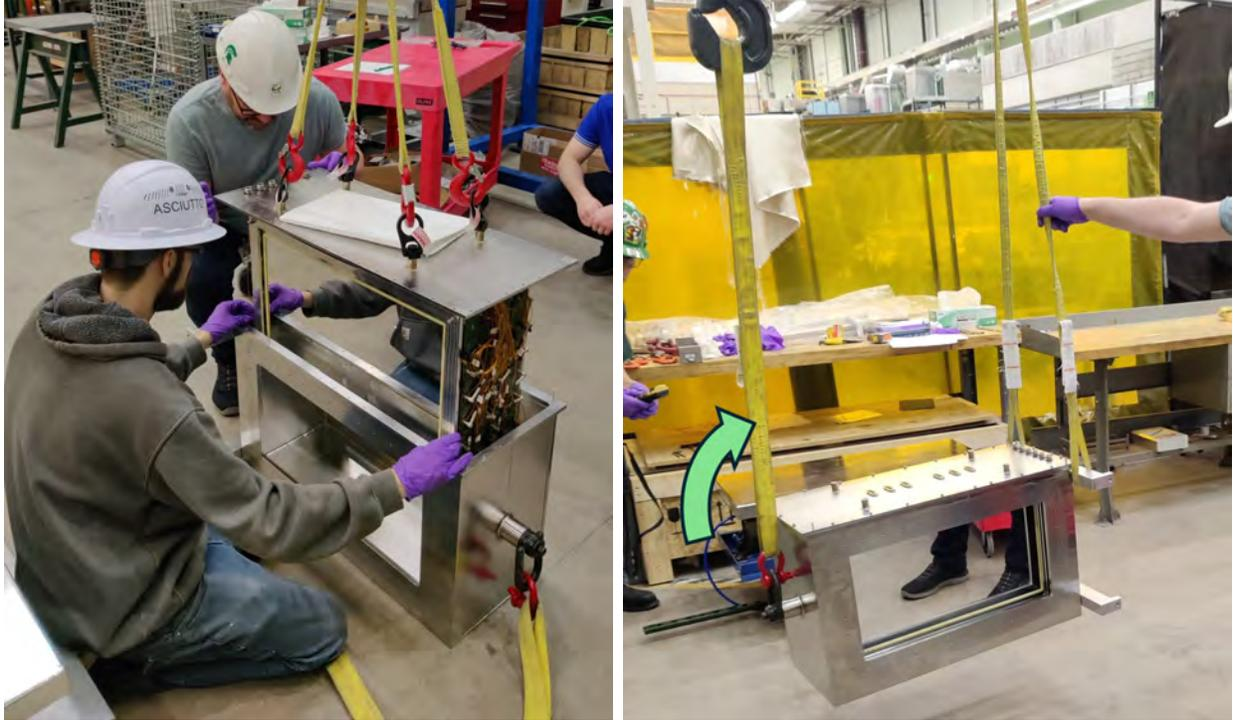
Figure 4.7: Left side: ELOSS optical readout (attached to lid) being lowered into the detector vessel. The crane connects to the four anchor points on the lid. Right side: one crane attaches to the top anchor point and another holds the legs of ELOSS (legs are for installation on a moving table discussed later). Lifting the top rotates the detector smoothly.
