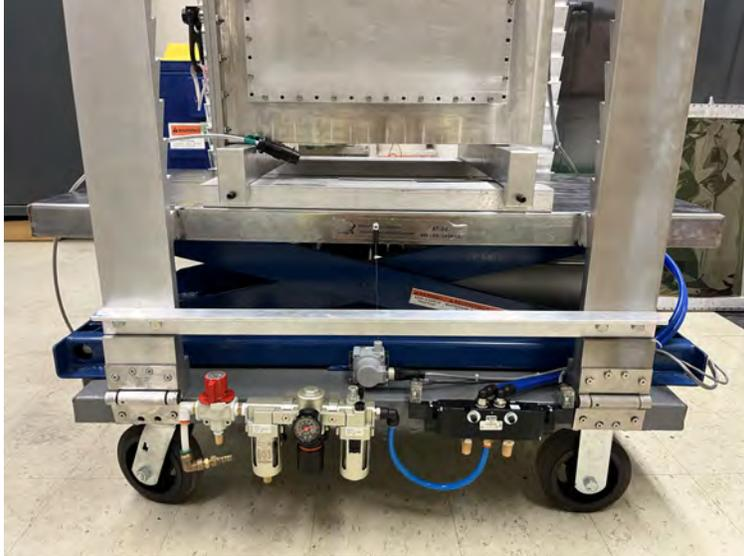
Figure 7.3: ELOSS Moving Table consisting of a pneumatic cylinder controlled scissor-lift for vertical motion and a motorized linear actuator mounted on the bottom of the truck platform with the wheels controlled the horizontal motion.
