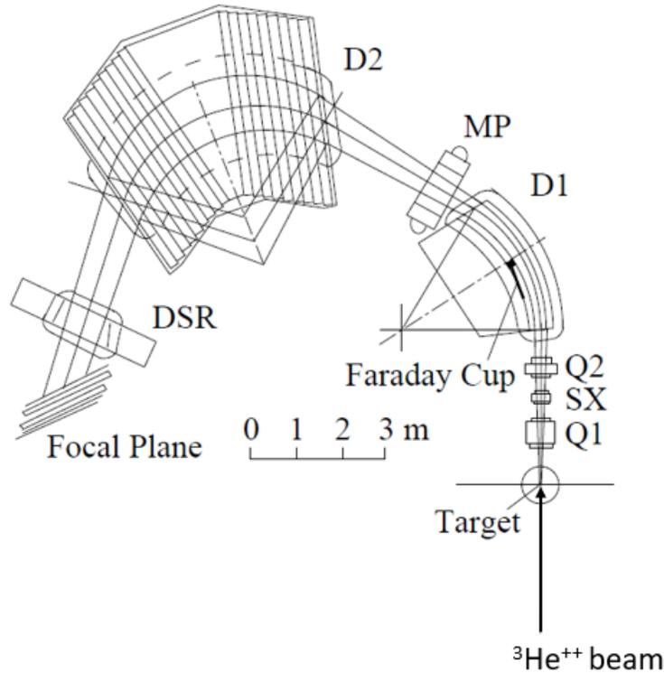
Figure 4.2 Schematic representation of the Grand Raiden Spectrometer set at  $0^\circ$ . The position and angle are measured in the focal plane detectors. The momentum vector of the ejectile is deduced, from which the excitation energy in the residual nucleus and scattering angles are determined. Figure modified from Ref. [131].
