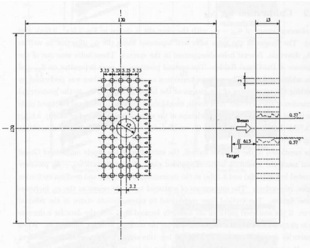
Figure 4.5 An example of the structure of sieve slit of the GRS for calibration of scattering angles. Figure taken from [135]
