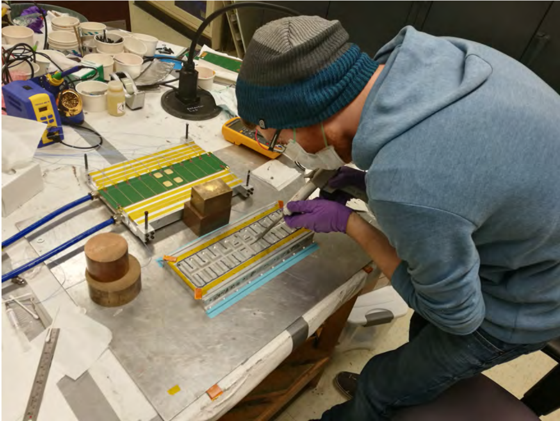
Figure 3.7 Picture taken during the gluing process. The anode is held level on a vacuum plate in preparation, while epoxy is applied to the aluminum base plate by the author of this dissertation. The vacuum plate was then lowered onto the bas plate to allow the epoxy to bond.
