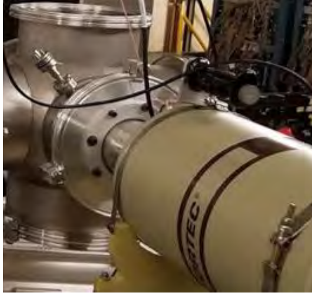
Figure 3.9 An external view of the HPGe detector. The liquid nitrogen Dewar can be seen.
