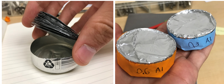
Figure 5.5 Constructed aluminum target designed to match the target densities of the powders to be tested.
