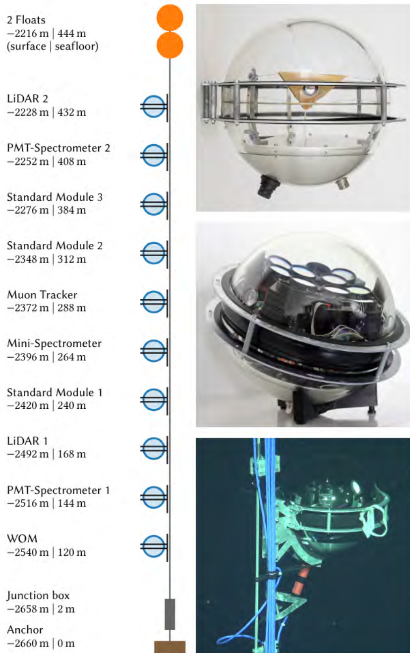
Figure 2.8: A sketch diagram of the STRAW-b mooring line(left), indicating the locations of all modules. Examples on the right show the housing glass sphere Standard Module (top right) and the PMT-Spectrometer (middle right and bottom right). Figure taken from [12]
