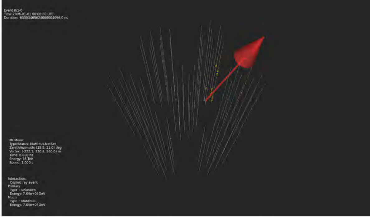
Figure 4.17: A screenshot of the event viewer of a simulated track event of 76 TeV that is estimated to have a visible length of 160 m in the detector volume.
