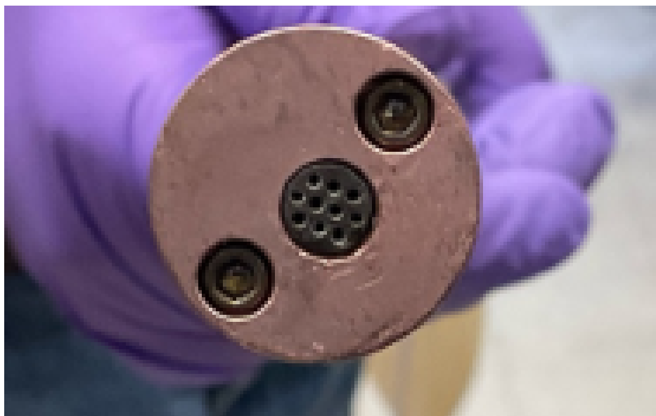
Figure 1.5 Copper head of the Low Temperature Oven (LTO). Oven exit is equipped with multiple holes. The screws on either side of the exit are used to attach the head to the oven shaft after loading the crucible.
