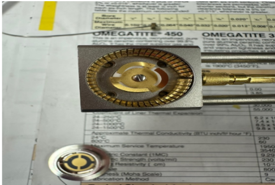
Figure 2.4 Inside view of the microbalance sensor. Three gold prongs make contact with the back of the crystal, which is held in place by a stainless-steel crystal holder. Gold springs circling the outside of the sensor hold the crystal holder in place and allow for easy access.
