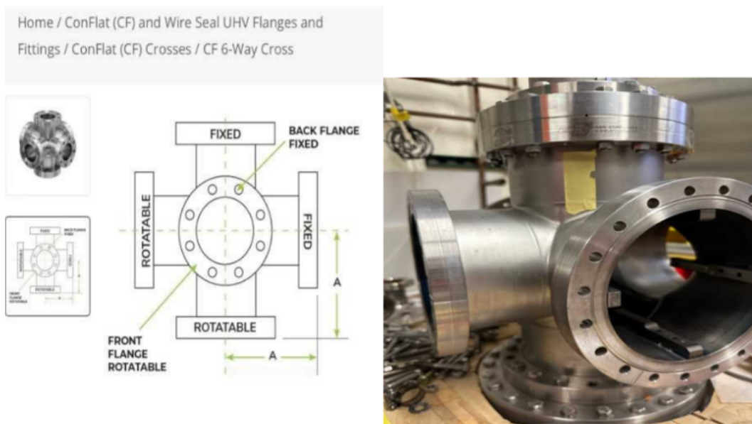
Figure 2.1 6-Way Cross UHV chamber from ANCORP. A variable from the schematic is in reference to the 6.56 inches of distance between midpoint and flange exit. Certain flange fittings are fixed or rotatable. Tube O.D. is 6 inches and the flange O.D. is 8 inches. Includes ConFlat flange capabilities.
