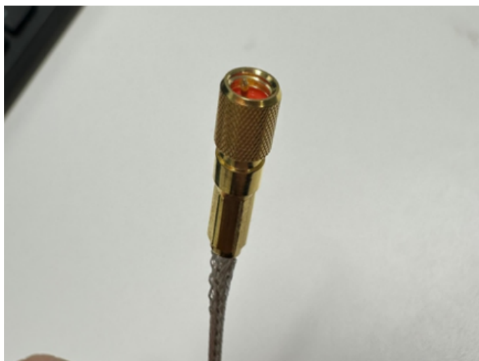
Figure 2.5 In-vacuum cable with gold-plated microdot connection. The inside wire tip component of the connection is crooked, causing the cable to not function properly.
