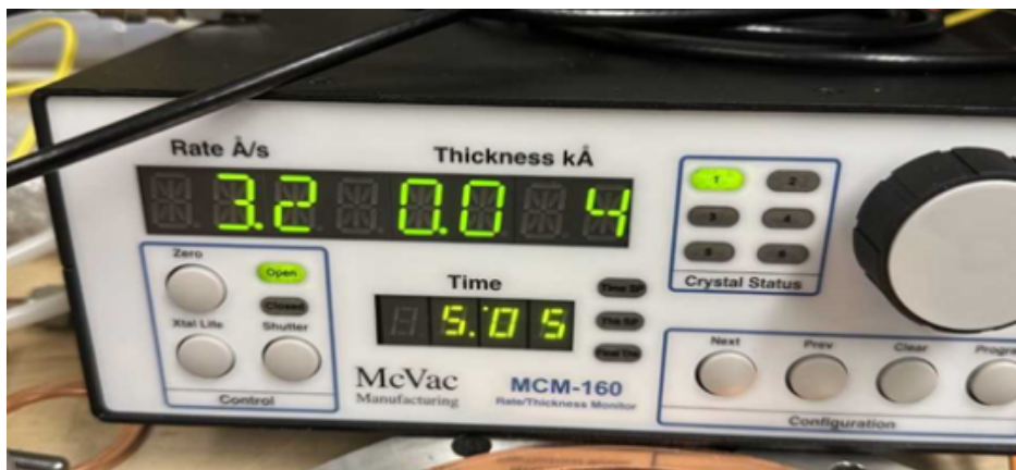
Figure 2.7 Monitor used for visualizing flux and mass readings from the quartz crystal. Important buttons include the “zero” and “xtal life”, along with the configuration buttons which allow for z-ratio and density adjustments for specific materials.
