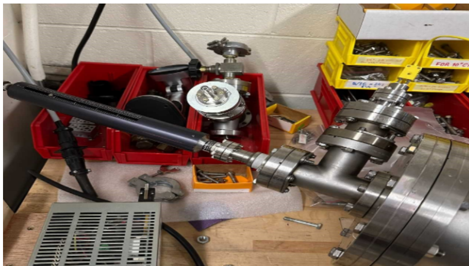
Figure 2.3 Linear feedthrough and type K thermocouple feedthrough joined with a 2 ¾" fitting. Results from this testing encouraged us to move along with the microbalance study, as the temperature recorded from this setup would be within a reasonable range for data acquisition with the microbalance.
