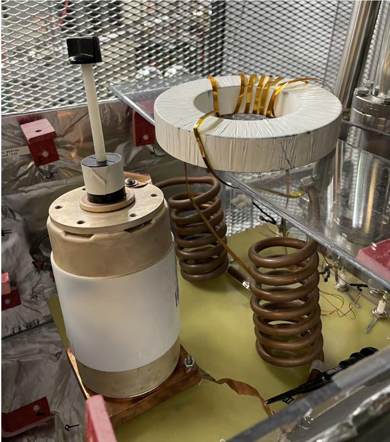
**Figure 3.26 Upgraded LC circuit for the cooler buncher.** The upgraded LC circuit is shown with the variable vacuum capacitor on the left and disc inductor on the top right. The impedance matching was achieved by a 1:49 step down transformer.
