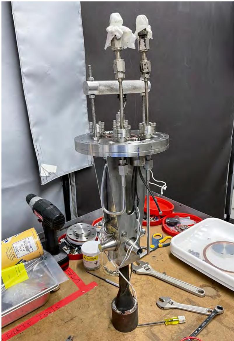
**Figure 3.28 CEC.** A photo of the CEC taken when the cell was removed from the beamline to be cleaned is shown. The cell usually hangs into the beamline to intersect with the ion path.
