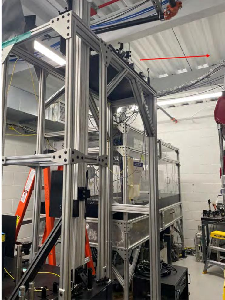
**Figure 3.15 BECOLA bridge.** A photo of the platform, nicknamed "BECOLA bridge", which sends laser light from the laser room to the beamline is shown. The red arrow indicates where the laser light travels.
