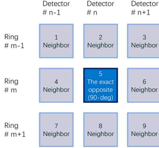
Figure 5.8: Definition of the relaxed coincidence condition including the neighbors of the opposite detectors.
