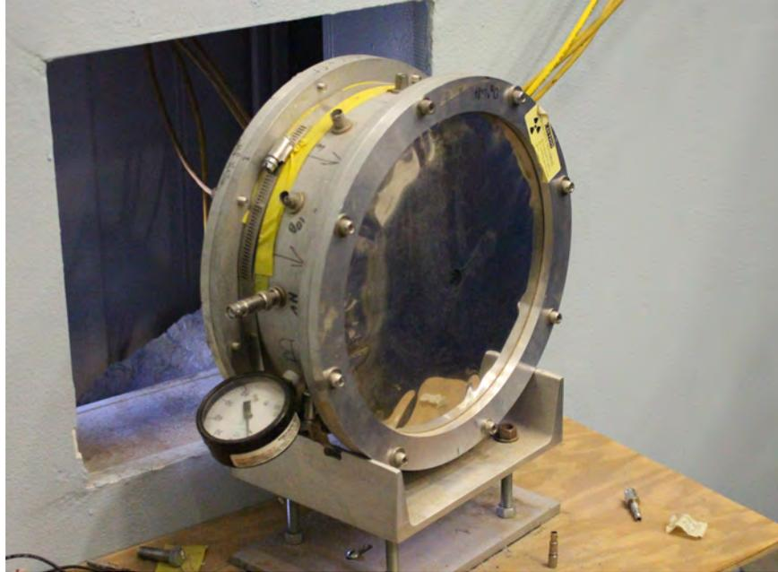
Figure 2.5: The fission chamber located downstream of Chi-NU/CoGNAC, 28.4 m away from the spallation target. The signals from the chamber were routed into the Chi-NU/CoGNAC DAQ. Neutrons pass through the rectangular cutout behind the fission chamber on their way to the 90 m station.
