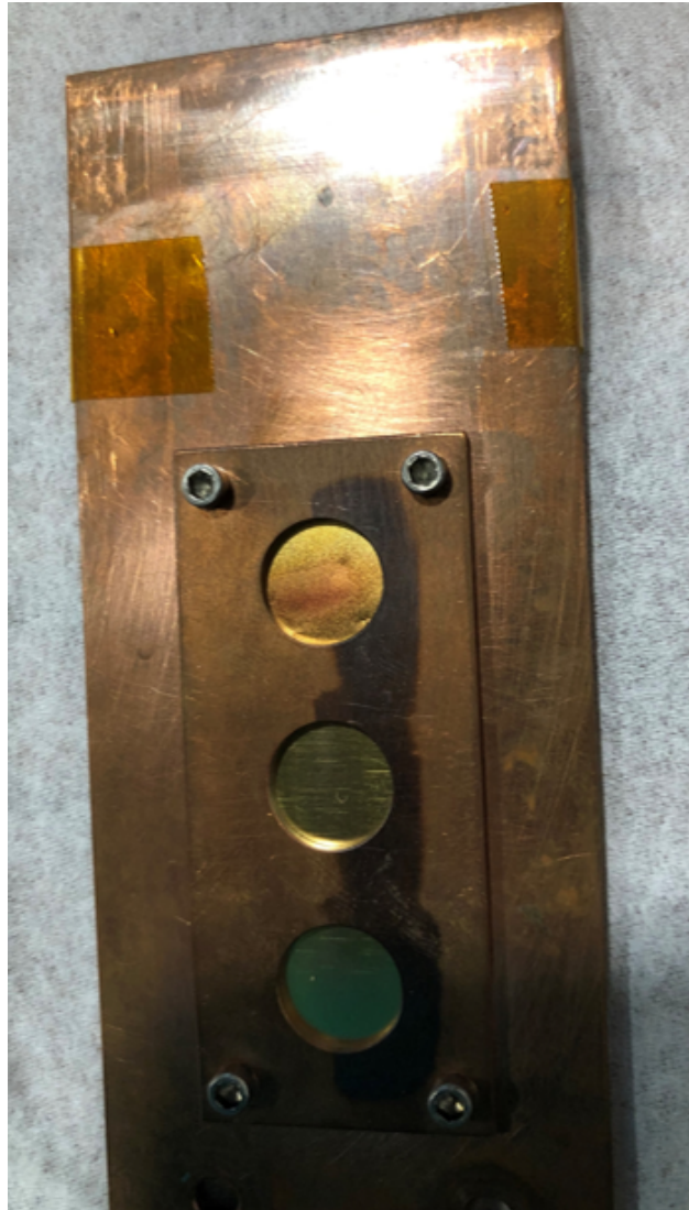
Figure 3.3 The targets on the target ladder in the configuration used in the experiment. The topmost target was produced at LLNL, and the lower two targets were produced at TRIUMF. The top two targets were used during the experiment.
