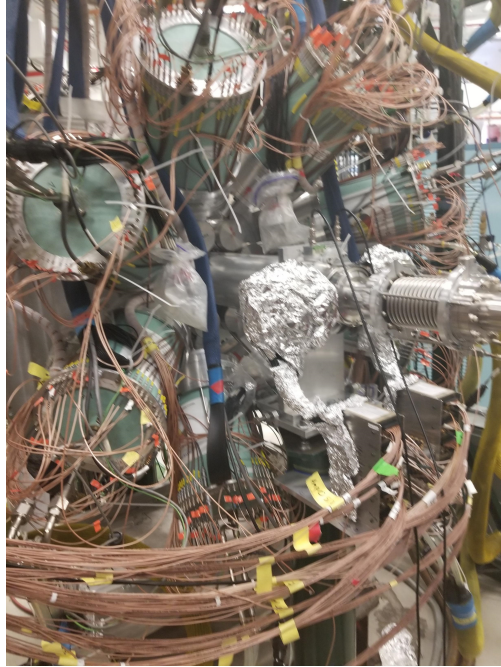
Figure 3.14: The upstream side of the experimental end station, showing the backward ring of SeGA and the silicon preamplifiers. Aluminum foil was used to provide shielding for the detector signals.
