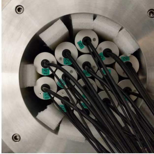
Figure 6.3: Setup of the 14 BGO array used for the dipole calibration runs. The flange is mounted on the JENSA chamber.
