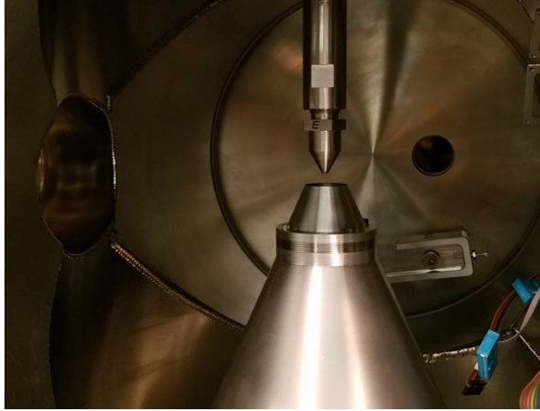
Figure 3.10: The JENSA nozzle and receiver installed in the ReA3 Hall. Beam direction is right to left.
