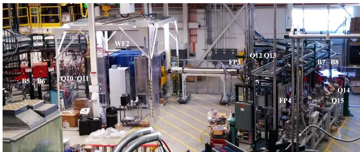
Figure 3.3: SECAR in the ReA3 Hall showing B5 up to the final focal plane.
