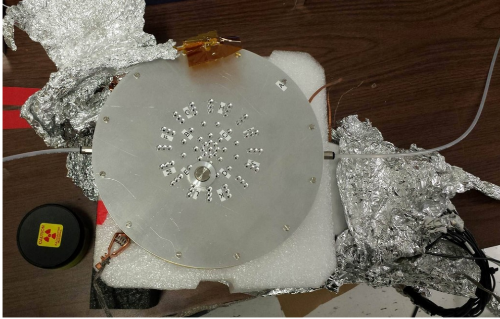
Figure 3.4: The MICROMEGAS being operated in “pancake” mode. By shorting the active volume of the gas, we were able to use an ^{55}\text{Fe} X-ray source to characterize the performance of individual detector pads.
