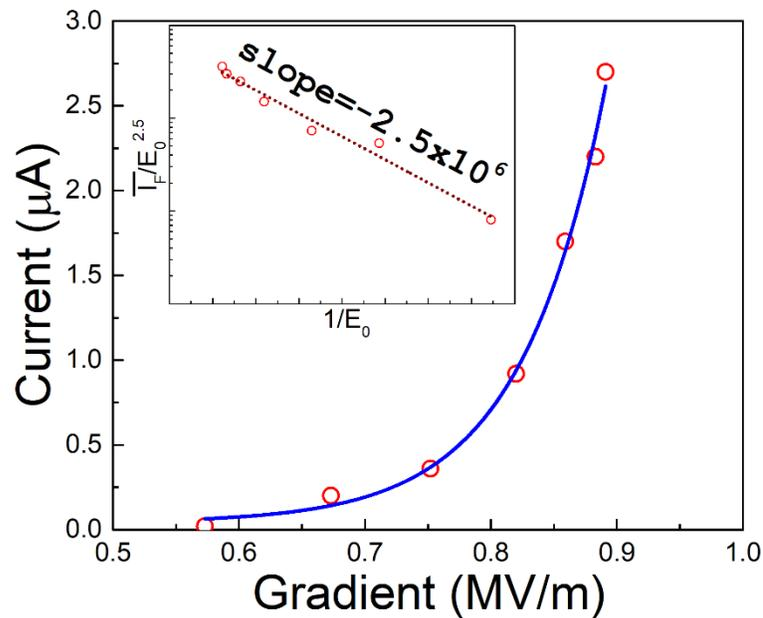
Fig. 1.2.1 UNCD cathode operated in a L-band SRF injector would turn on field at 0.6 MV/m [31]. AIP Publishing grants a license for all orders.
