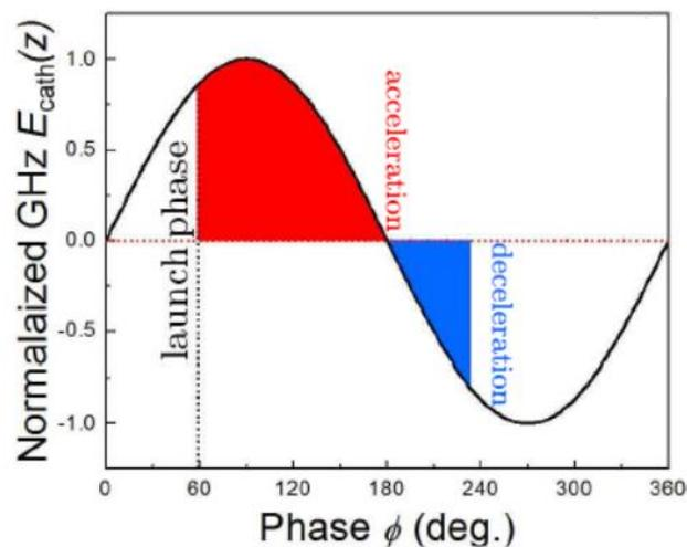
Fig. 1.1.3 FEC RF phase window from J. Qui and S. Baryshev, IEEE Transactions on Electron Devices 65, 1132 (2018) [15]. The IEEE does not require individuals working on a thesis to obtain a formal reuse license
