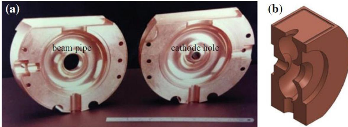
Fig. 2.1.1 (a) transverse cross-sectional photo of ACT gun showing the beam aperture and the cathode holder. Photo was taken before brazing the two sections of the cavity into one part. (b) shows a longitudinal cross-section of the 3D model of the ACT gun [1]. Ability to reprint figure under the license number **5192550991050**
