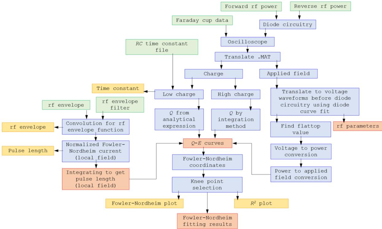
Fig. 3.2.1 FEbeam’s workflow map showing how the data processing algorithm (in blue) takes the raw data from input files (in green) to the output data (in red) and the output figures (in yellow) [1]. AIP Publishing grants a license for all orders.
