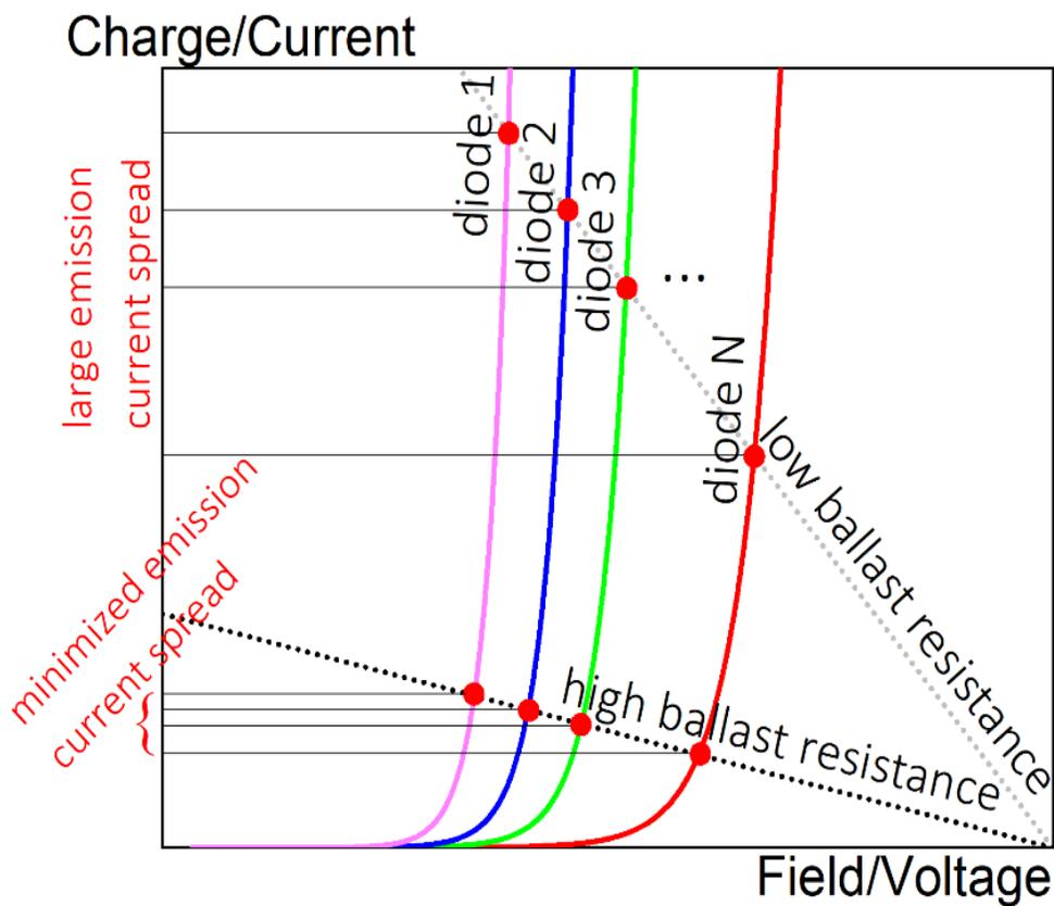
Fig. 4.3.7 Simplified loadline representation of the ballast resistance effect.
