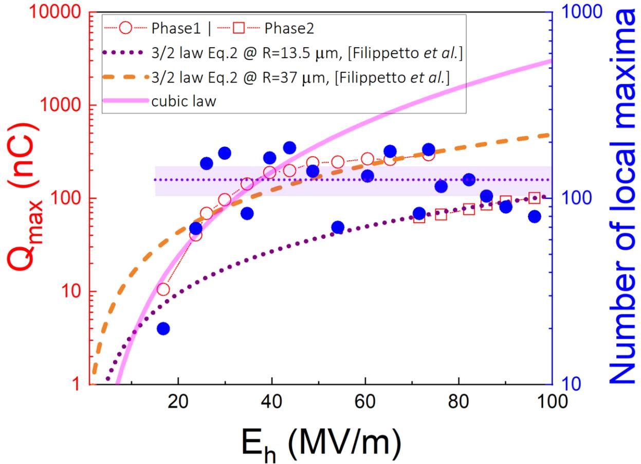
Figure 4.2.1 Maximum charge and the number of emitters determined at the maximum of every conditioning Q-E curve as functions of  $E_h$ . The purple horizontal area represents one standard deviation around the mean value of the emitter number count [33]. It is not necessary to obtain permission to reuse this article or its components as it is available under the terms of the [Creative Commons Attribution 4.0 International](https://creativecommons.org/licenses/by/4.0/) license.
