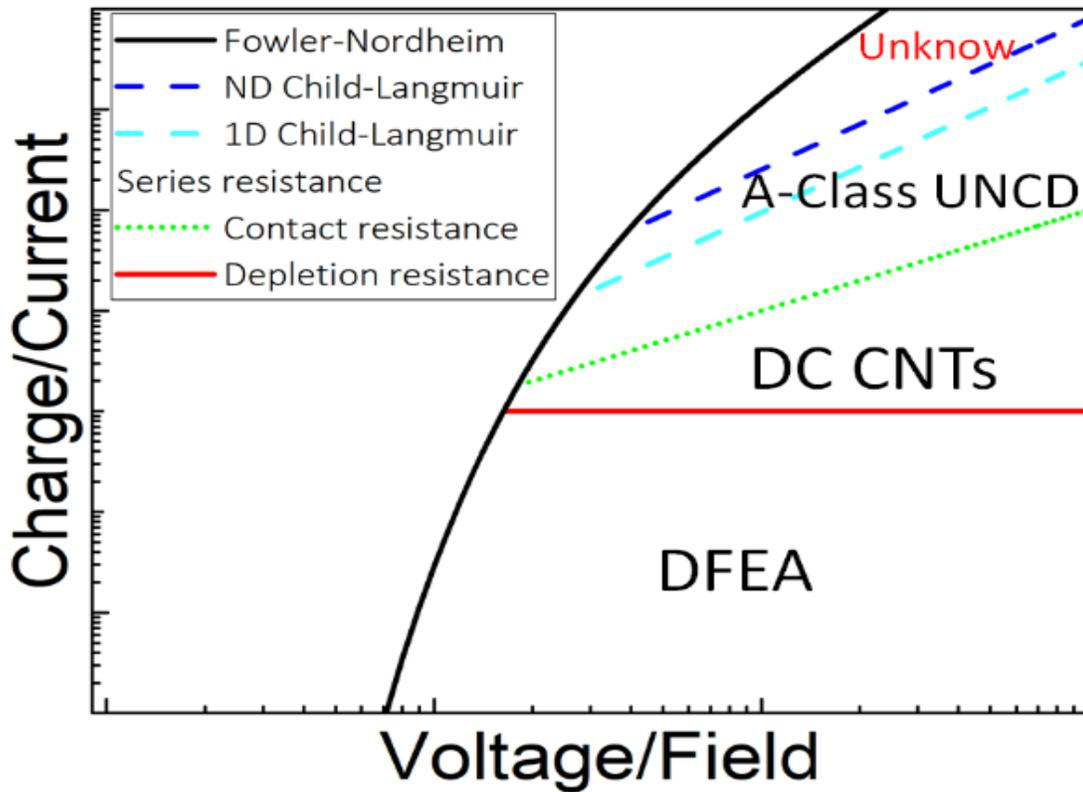
Fig. 4.3.8 Concept map showing the different regions of field emission dynamics under high charge high gradient conditions.
