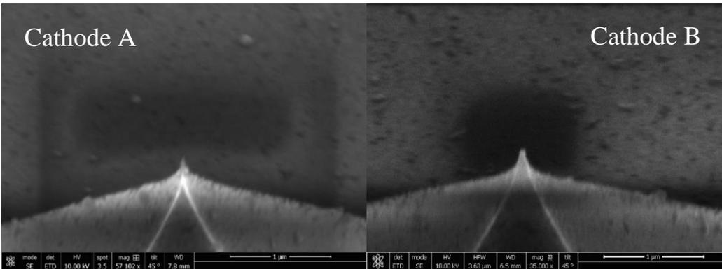
Fig. 4.3.1 SEM image of a single emitter pyramid showing the sharpness of the emitter tip for cathode A and cathode B.
