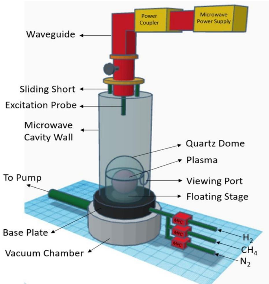
Fig. 1.2.5 Diagram of the UNCD growth chamber used at Michigan State University and the Fraunhofer Institute [38]. This figure has been approved to be reprinted in accordance with approval from the author Tanvi Nikhar MS
