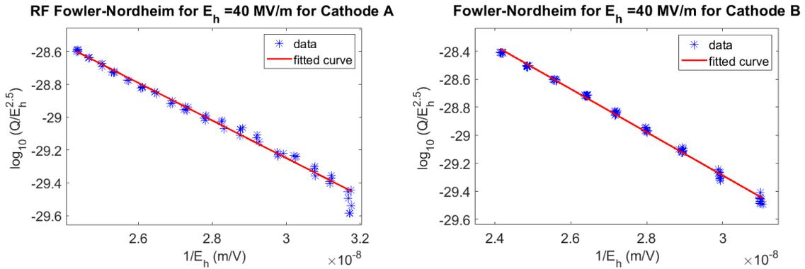
Fig. 4.3.3 FN plots for cathode A and cathode B both conditioned to 40 MV/m showing ideal linearity.
