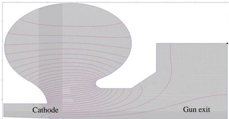
Fig. 2.1.2 E field map line concurrence of ACT gun concavity of field lines shows where the field is most off-axis [1]. Ability to reprint figure under the license number **5192550991050**.
