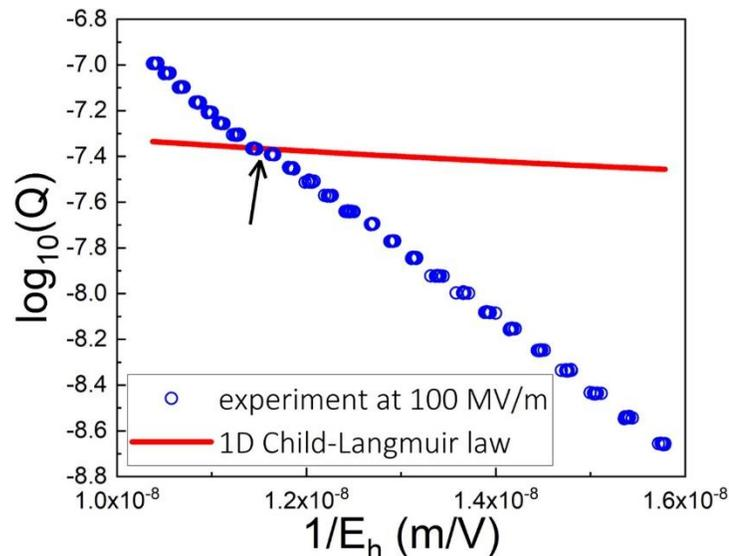
Fig. 4.2.2 Millikan plot for 100 MV/m (red) showing the parallel shift denoted with an arrow and is indicative of a space charge dominated regime that differs from the Child Langmuir law (blue). Additional Millikan plots can be seen in [Appendix B](#). It is not necessary to obtain permission to reuse this article or its components as it is available under the terms of the [Creative Commons Attribution 4.0 International](#) license.
