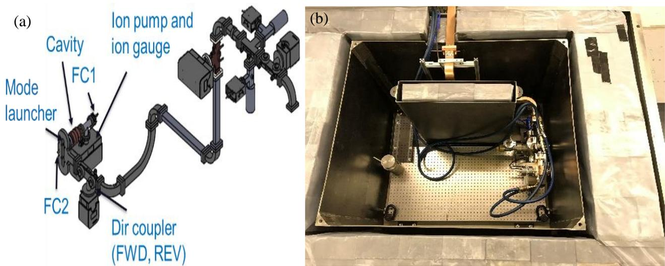
Fig. 3.4.1 (a) CAD model of waveguide components and diagnostics, (b) a photograph of the current state of the part of the CERF-NM facility in lead box enclosure. All JACOW conference proceedings are published under the Creative Commons Attribution 3.0 license (CC-BY 3.0) to copy and redistribute the material in any medium or format.
