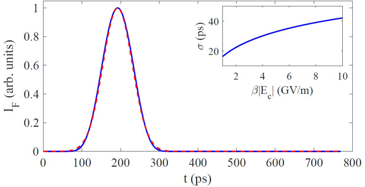
Fig. 3.2.6 Emission profile within one rf cycle based on Eq. 3.1.1 (blue solid line) and its Gaussian distribution approximation (red dashed line). Inset: The standard deviation of the Gaussian distribution as a function the maximum microscopic cathode field [1]. AIP Publishing grants a license for all orders
