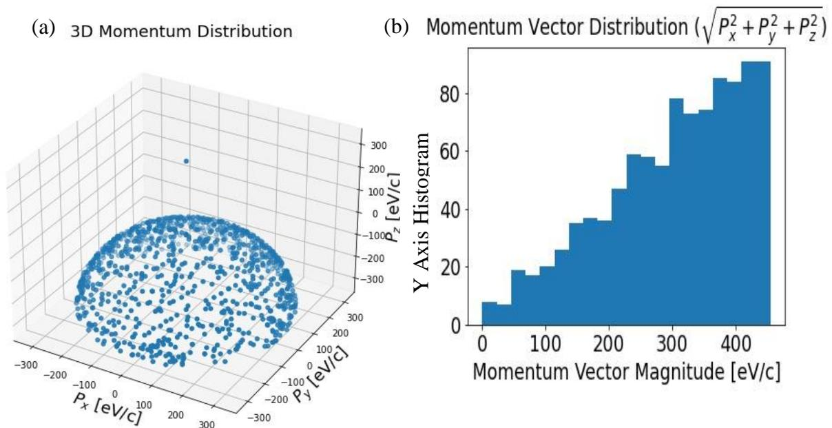
Fig. 3.1.1 (a) isotropic distribution in momentum space. The single point above the sphere is the test particle where all of the momentum is in the z direction; (b) the distribution for the magnitude of the momentum vector [2].
