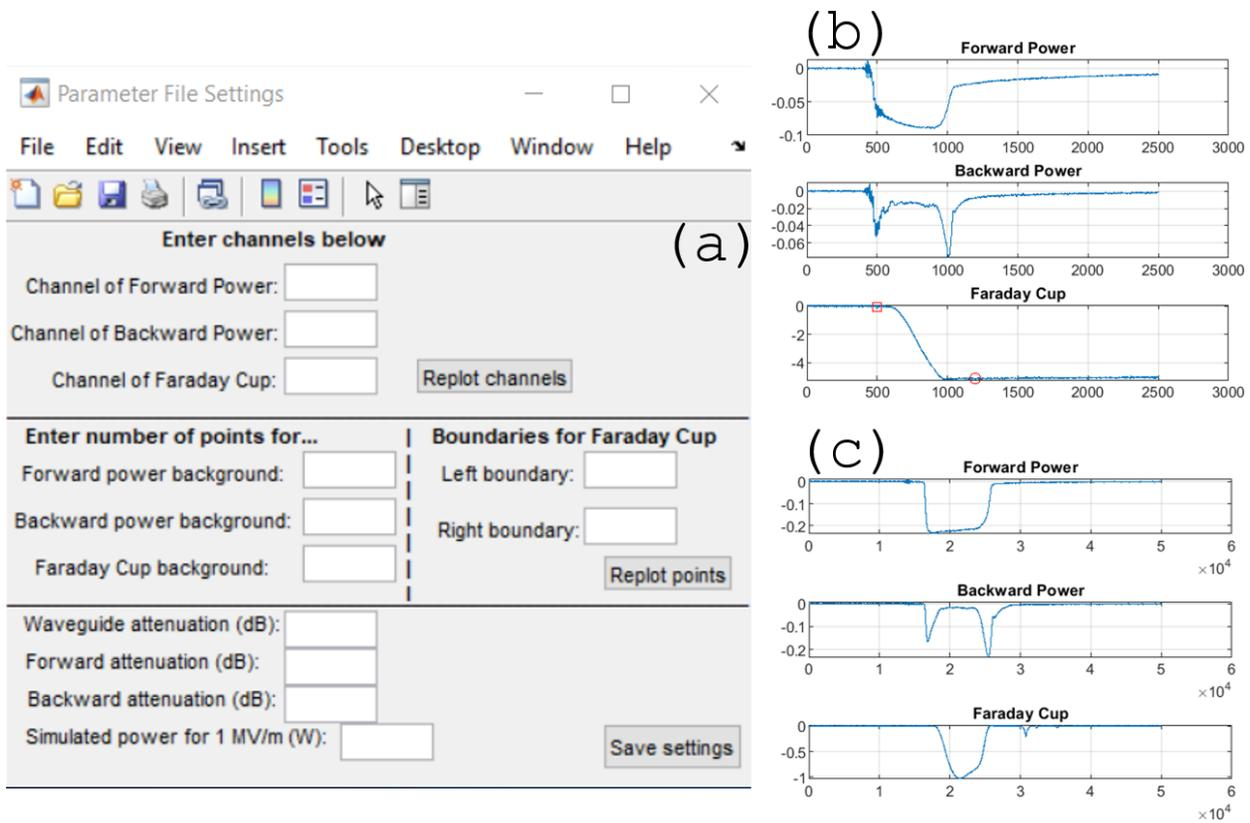
Fig. 3.2.5 (a) Parameter File Settings for entering the rf parameters to calculate the Q-E curves; (b) waveforms for a low charge scenario; (c) waveforms for a high charge scenario. Red marks denote the region that was considered in the Faraday cup to calculate the charge. AIP Publishing grants a license for all orders
