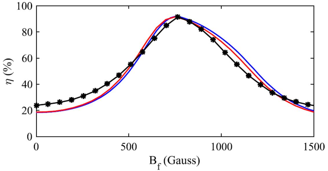
Fig. 2.1.5 Capture ratio for UNCD for  $E_h= 43$  MV/m (black line) compared with simulation values for capture ratio of  $|E_h|$  (red line) and  $E_{h\max}$  [2]. It is not necessary to obtain permission to reuse this article or its components as it is available under the terms of the [Creative Commons Attribution 4.0 International](https://creativecommons.org/licenses/by/4.0/) license.
