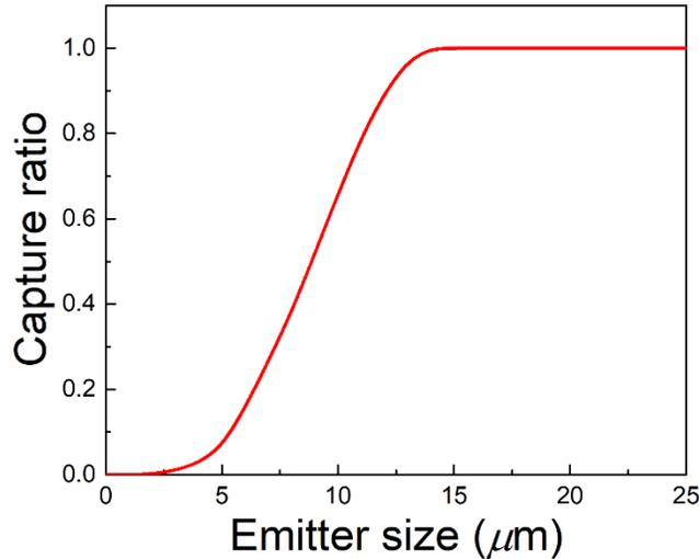
Fig. 4.3.5 Faraday cup capture ratio at  $E_h=40$  MV/m as a function of emitting tip size.
