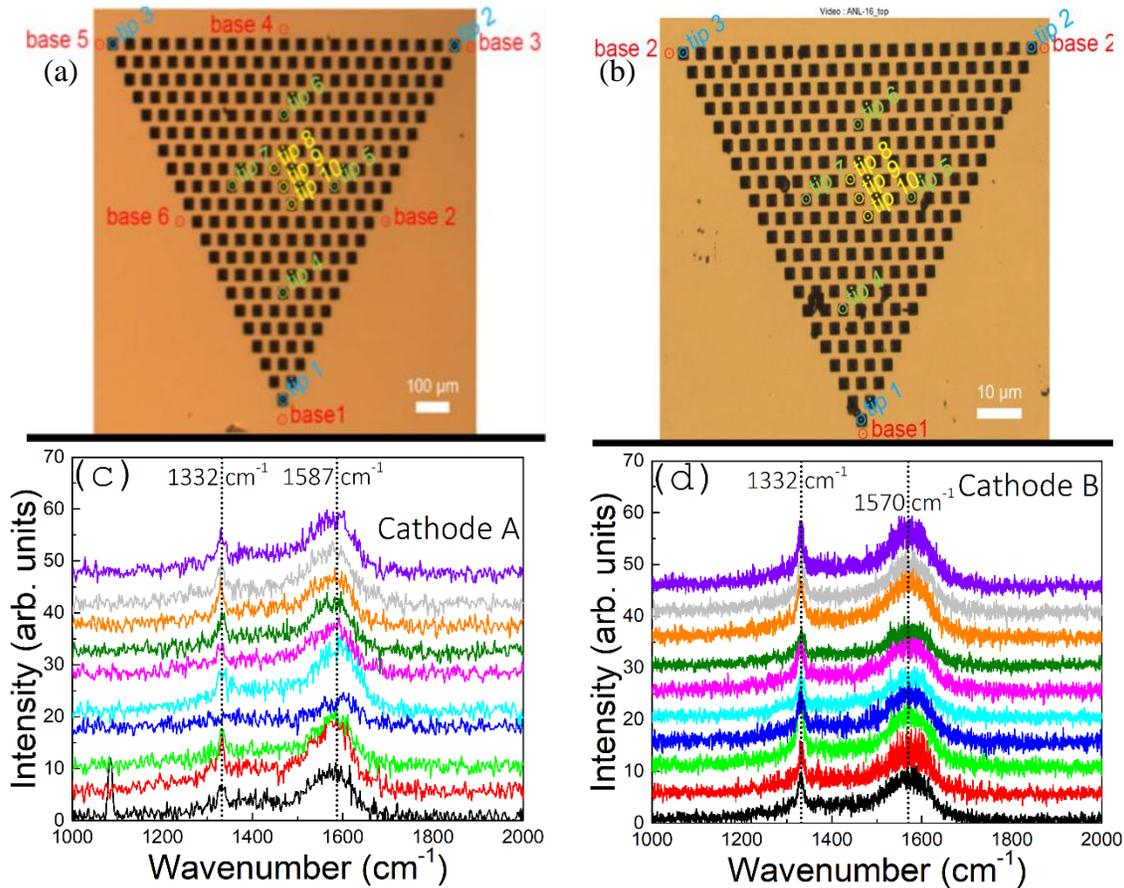
Fig. 4.3.6 Raman spectrum comparison between cathode A and cathode B, locations of tips (a) measured for Raman spectrum seen in (c) for cathode A. Likewise locations of tips (b) measured for Raman spectrum seen in (d) for cathode B.
