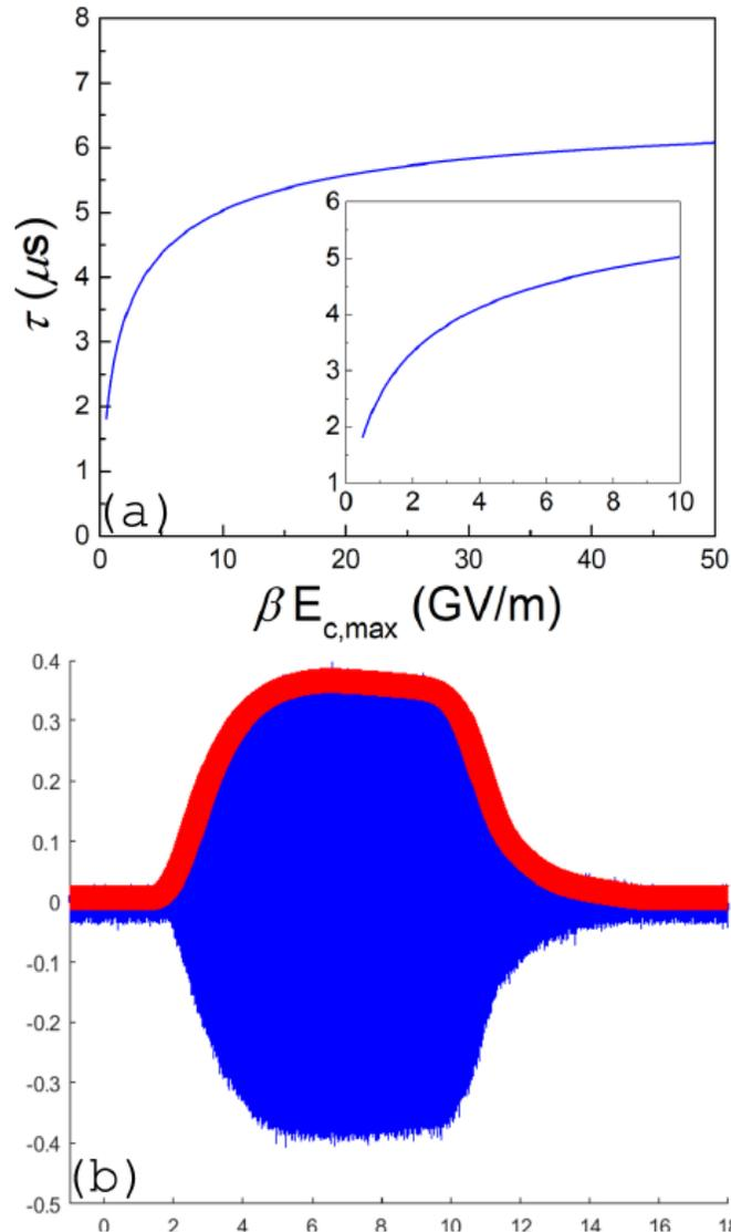
Fig. 3.2.8 The emission pulse length ( $\tau$ ) as a function of the local field plotted in the entire fitting range from 0 to 50 GV/m, inset is a zoom-in view of the pulse length within the physically meaningful local field range, from 0 to 10 GV/m. (b) In red is the rf envelope after frequency filter was applied, in blue is the actual pulse measured using pickup in the gun. AIP Publishing grants a license for all orders
