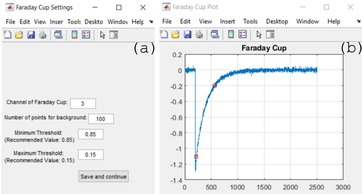
Fig. 3.2.4 (a) Faraday Cup Settings display interface for selecting the time constant for the low charge case. (b) Plot where red square and circle denote the location of the minimum and maximum threshold values corresponding to 90% and 10% of the maximum value [1]. AIP Publishing grants a license for all orders
