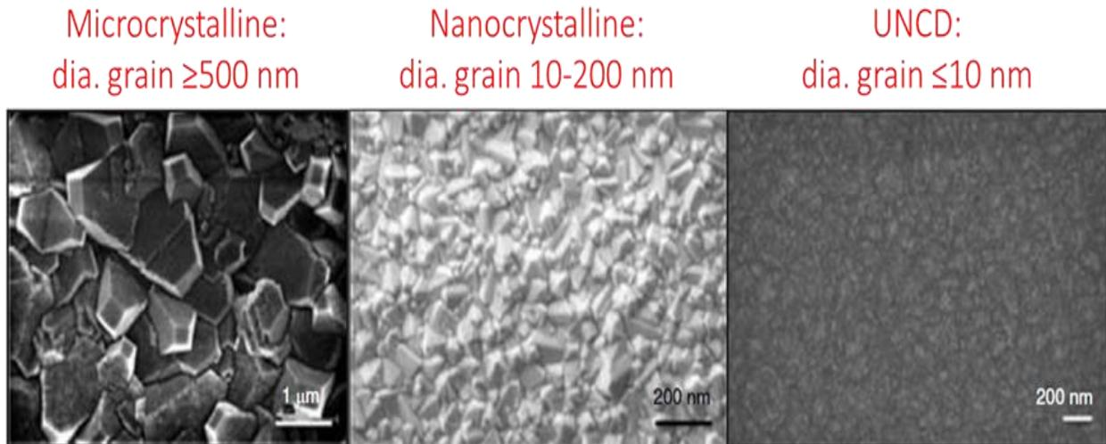
Fig. 1.2.3 SEM images showing the relative grain size between different forms of polycrystalline diamond being that of micro, nano, and UNCD from [34]. Ability to reprint figure under the license number **5192220196519**
