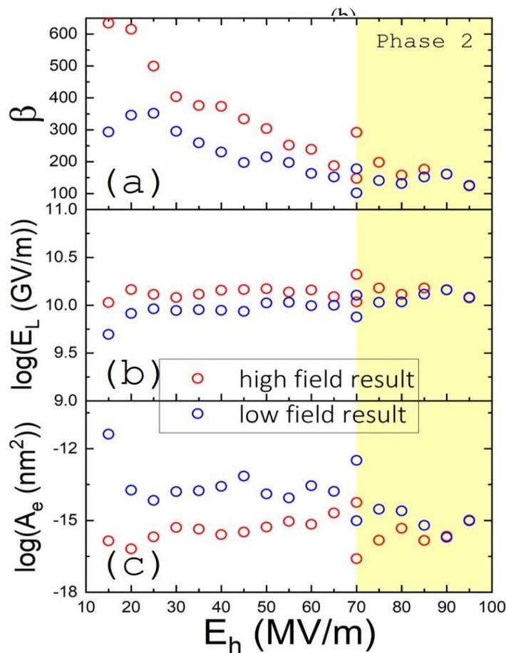
Fig. 4.1.6 Field emission conditioning parameters: (a) field enhancement factor, (b) local field on the cathode surface, and (c) effective emission area for both the FN-like (low field) and non-FN (high field) regions [33]. It is not necessary to obtain permission to reuse this article or its components as it is available under the terms of the [Creative Commons Attribution 4.0 International](https://creativecommons.org/licenses/by/4.0/) license.
