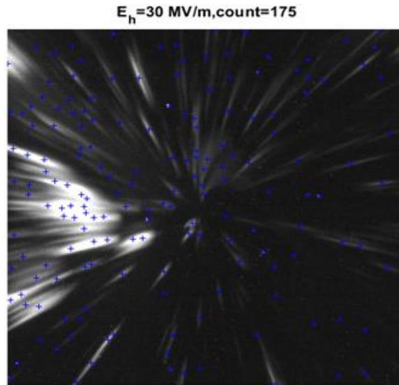
Fig. 3.3.2 Illustration of closely packed emitters extracted from data for A-class UNCD FECs from the experiment outlined in CH4.
