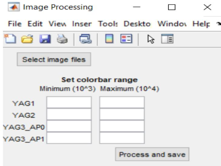
Fig. 3.3.1 FEpic inside of FEMaster options for selecting minimum and maximum threshold for image visualization. Options include all three YAG on the ACT and YAG3 having two options one with and without the aperture.
