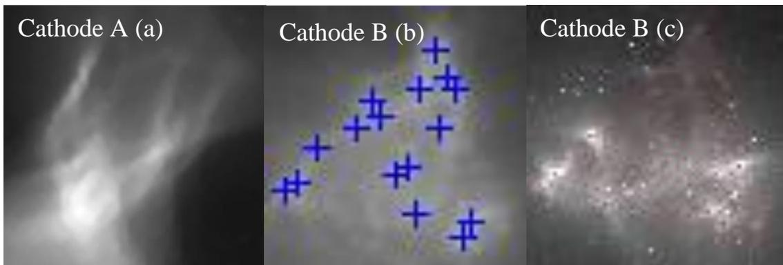
Fig. 4.3.4 Image taken on YAG3 at 40 MV/m for cathode A and cathode B. Cathode A showing no pattern beam and a large electron cloud due to space charge domination. Cathode B showed a pattern of emission and local maximum determined using FEpic blue crosses in center picture (not to scale); (c) Overlay of the initial DFEA pattern times a magnification factor of 12 (red dots) and the local maximums determined from FEpic (blue). Marker size is to scale at  $E_h=30$  MV/m.
