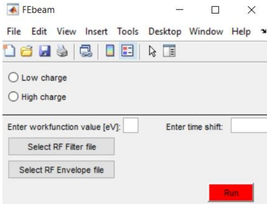
Fig. 3.2.3 The main interface of FEbeam. The top portion sets the rf parameters to translate the raw data into Q-E curves. AIP Publishing grants a license for all orders
