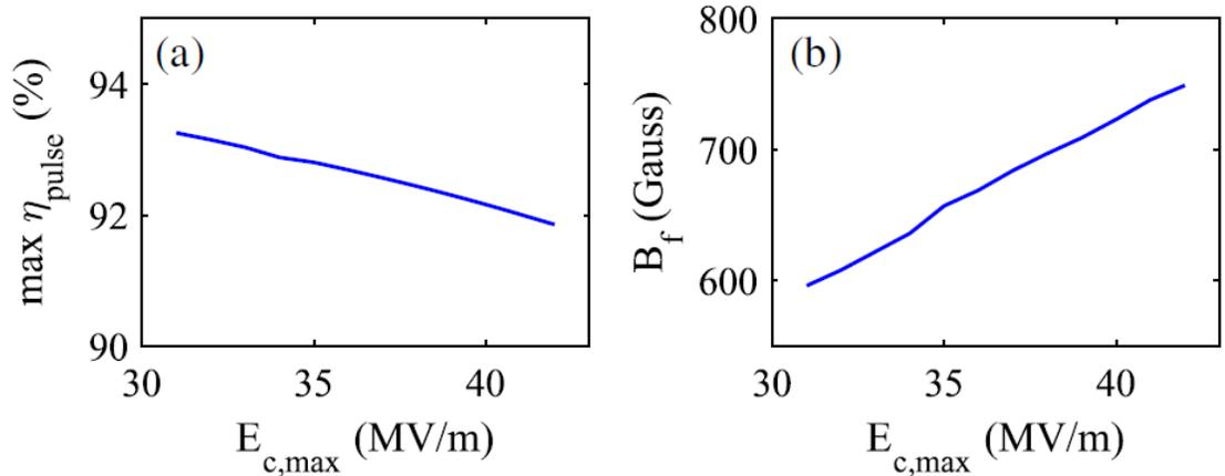
Fig. 2.1.6 (a) maximum capture ratio as a function of conditioning field  $E_c$  and the corresponding optical magnetic field of the focusing solenoid on the ACT beamline (b) [2]. It is not necessary to obtain permission to reuse this article or its components as it is available under the terms of the [Creative Commons Attribution 4.0 International](https://creativecommons.org/licenses/by/4.0/) license.
