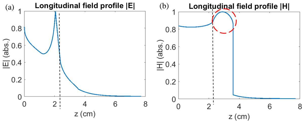
Fig. 2.1.3 (a) ACT field profile for the magnitude of the electric field, (b) magnetic field where dashed line represents the exit of the gun.
