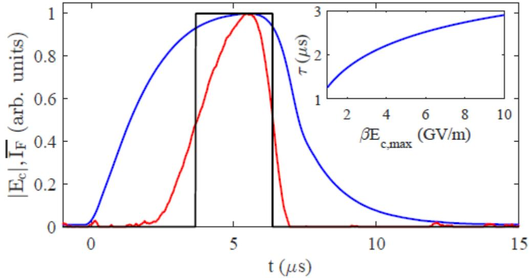
Fig. 3.2.7 Blue: the normalized cathode field amplitude  $|E_c(t)|$  measured by the rf pickup. Red: the predicted average emission current  $I_F(t)$  by Eq. 9. Black: the square pulse approximation of the emission profile. Inset: The width of the square emission profile as a function of  $\beta E_{c,max}$ . Reproduced from Ref.3. AIP Publishing grants a license for all orders
