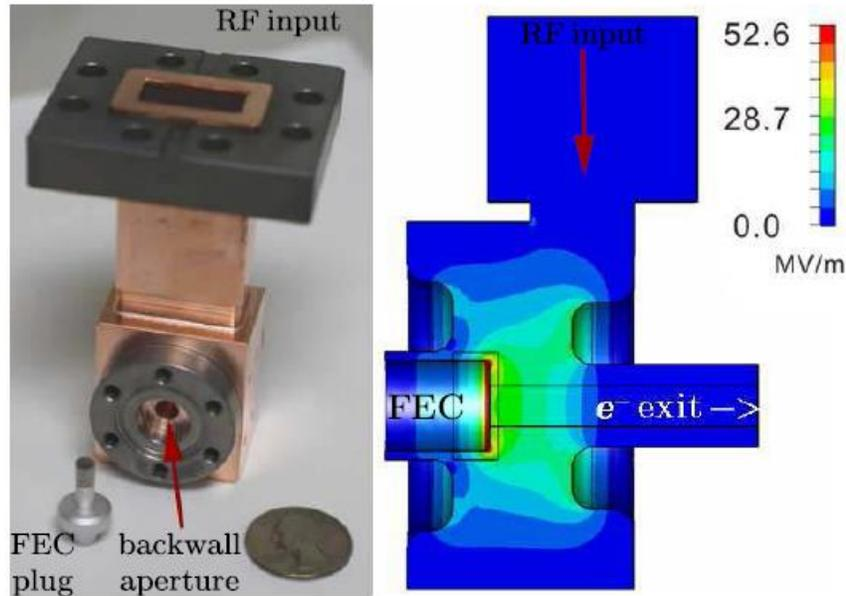
Fig. 1.2.2 copper normal conducting X-band injector with cathode plug and field map using a UNCD field emission cathode [33]. The IEEE does not require individuals working on a thesis to obtain a formal reuse license
