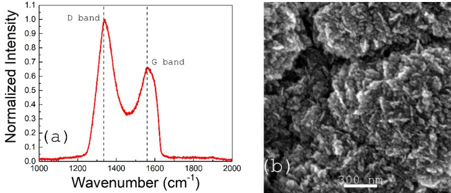
Fig. 4.1.1 Raman spectrum and SEM micrograph of as-grown sample [33]. It is not necessary to obtain permission to reuse this article or its components as it is available under the terms of the [Creative Commons Attribution 4.0 International](https://creativecommons.org/licenses/by/4.0/) license.
