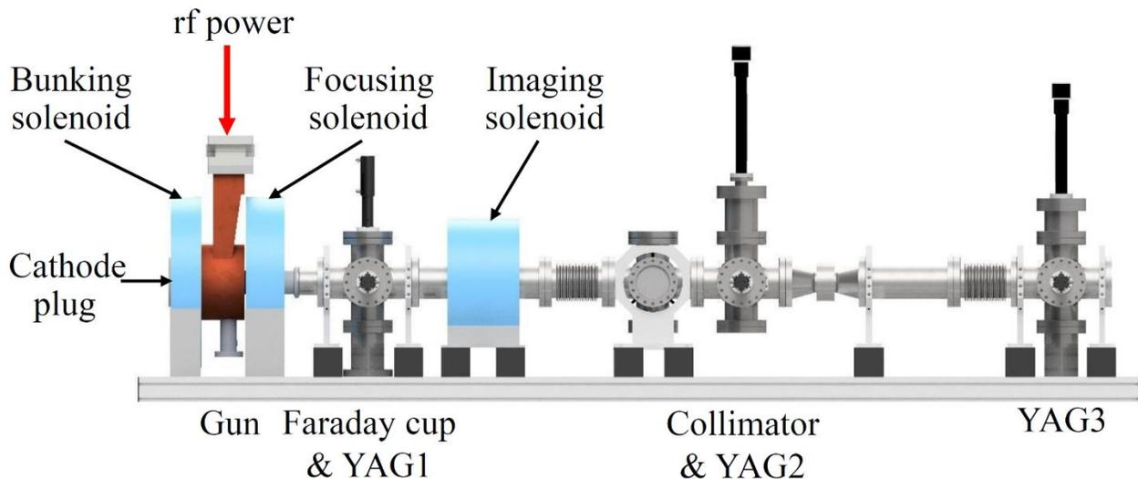
Fig. 2.1.4 Beamline diagram for the ACT showing all three of the solenoids and the location of the cathode with respect to the rest of the beam line and the three imaging stations. Not shown is the RF system before the gun [2]. It is not necessary to obtain permission to reuse this article or its components as it is available under the terms of the [Creative Commons Attribution 4.0 International](https://creativecommons.org/licenses/by/4.0/) license.
