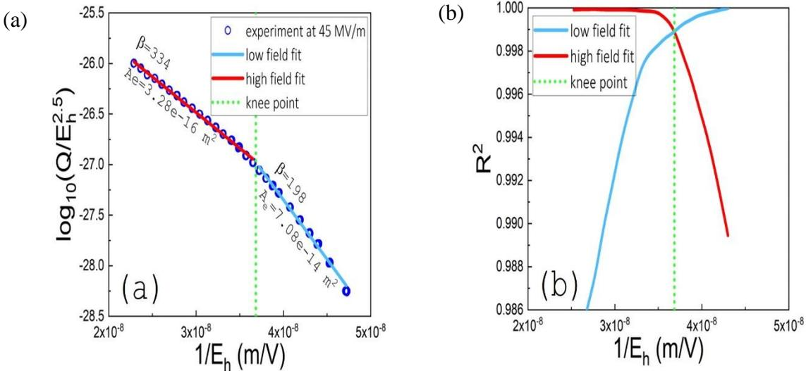
Fig. 4.1.5 (a) FN plot and (b)  $R^2$  plot exemplified for 45 MV/m. For all FN plot [Appendix B](#). [33] It is not necessary to obtain permission to reuse this article or its components as it is available under the terms of the [Creative Commons Attribution 4.0 International](#) license.
