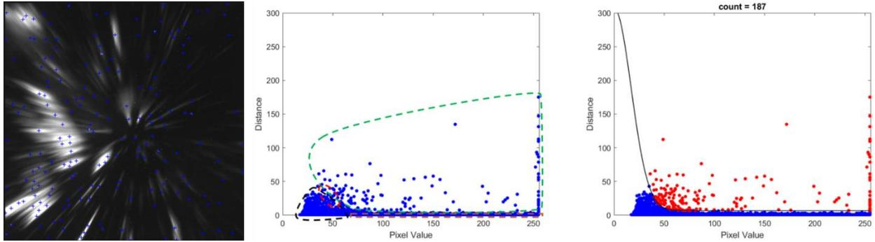
Fig. 3.3.3 (a) example of image processing results. (b) decision plot green line shows actual emitters, black line shows the noise, and red line shows the undefined region that is a mixture of noise emitters and actual emitters. (c) machine learning algorithms final decision for decision boundary Gaussian fitting function.
