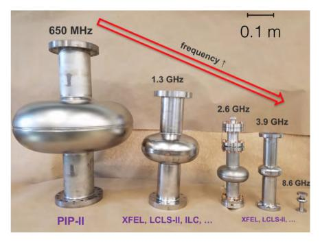
Figure 1.16: Cavity size comparison for different frequencies.
