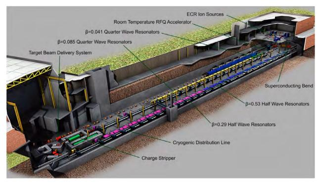
Figure 1.6: Layout of FRIB driver accelerator.
