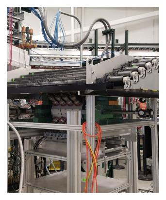
Figure 3.4: The SuNSCREEN detector sitting above the SuN detector from the experiment measuring the  ${}^{84}Kr(p,\gamma){}^{85}Rb$  cross section. The green bricks are lead bricks to help reduce background. The beam went through the center of SuN from left to right.
