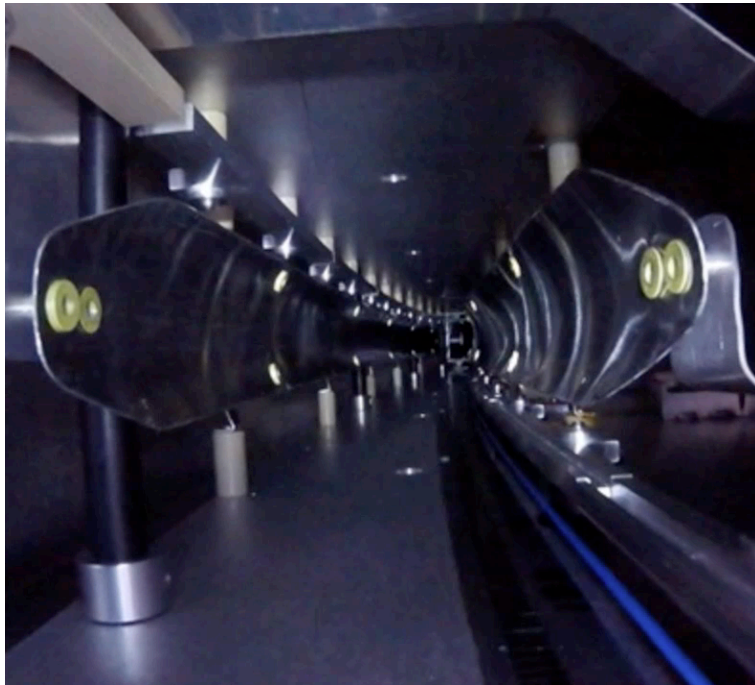
Figure 3.9: Transverse view of a kicker station. The plate geometry is designed to maximize current-to-field conversion in the storage region.
