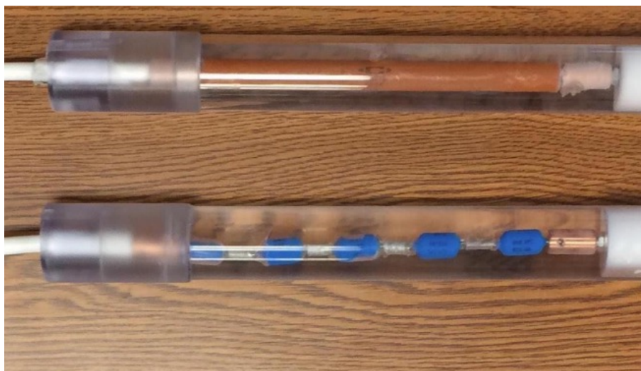
Figure 3.62: Single-CADDOCK high-voltage resistor (top) and chain of potted HV resistors (bottom). Two of the latter resistors became damaged during Run-1.
