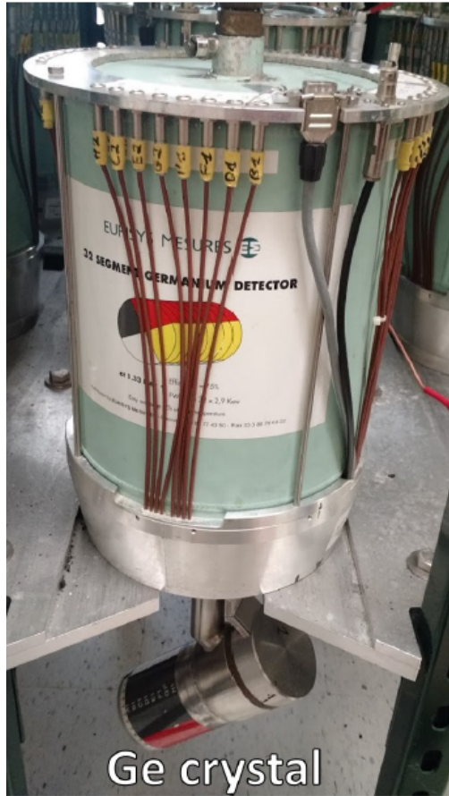
Figure 3.15: A single SeGA detector. The large green cylinder is the liquid-nitrogen dewar. The germanium crystal is located in the aluminum housing at the bottom of the photo. Figure from [108].
