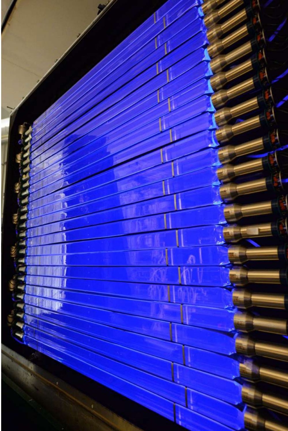
Figure 2.11: One of LANA walls is illuminated with ultra-violet light after the front aluminum cover is removed.
