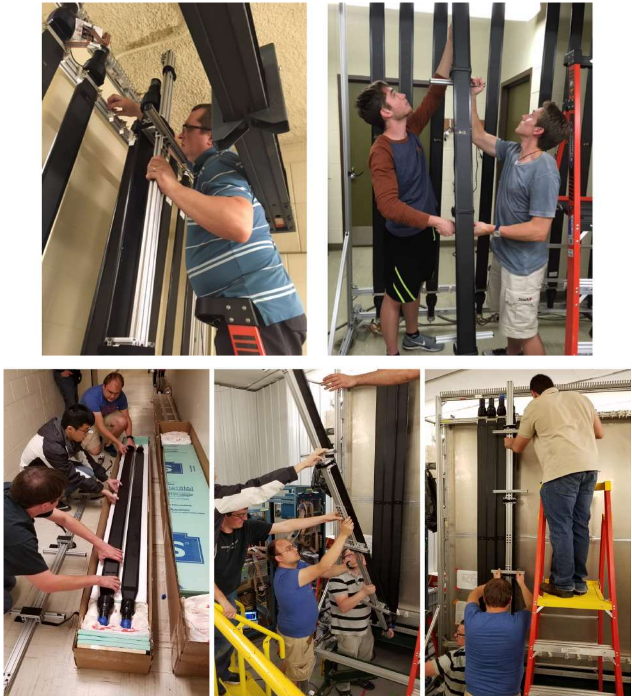
Figure 2.21: (top left panel) Professor Chajecski is testing the Charged-Particle Veto Wall frame. (top right panel) Undergraduate students from Western Michigan University and Michigan State University are moving Veto Wall bar. (bottom left panel) Veto Wall bars are being taken out from shipment packages. (bottom middle and right panel) NSCL and WMU researchers are installing the Charged-Particle Veto Wall in front of LANA.
