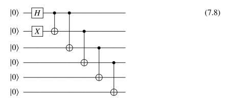
The first two rows prepare the Bell-state  $\left|\psi^{+}\right\rangle=(\left|01\right\rangle+\left|10\right\rangle)/\sqrt{2}$  and each subsequent pair of CNOTs "copies" the state of each term of the Bell-state and adds it onto that term.
