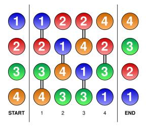
Figure 5.2: (Color online) Pictorial representation of the swap network used in our simulation in the case of N = 4 neutrinos.
