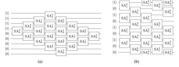
Figure 4.4: a) Linear particle-hole swap network (lphsn) for 4-particle, 5-hole system. b) Circular particle-hole swap network for 4-particle, 5-hole system (cphsn). See Figure 4.5 for schematic representation.
