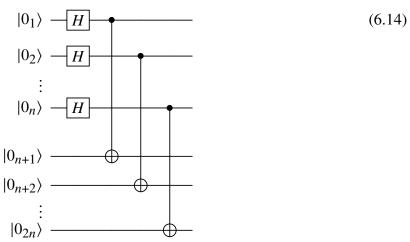
where the column of n Haddamard gates H places the top half of the qubits in the equal superposition of the states of  $H_n$  while the ladder of CNOT gates "copies" each state of top half of the qubits to the state of the bottom half, maximally entangling the two sets of qubits. Note that this is simply n copies of the quantum circuit that prepares  $|\Phi^+\rangle$ , (6.8) with  $|q_0q_1\rangle = |00\rangle$ . The proof of the maximum entanglement of  $|\phi_n^+\rangle$  is given below:
