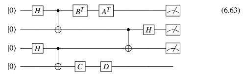
The entanglement swapping identity then tells us that, with a probability of 1/4, measuring the middle two qubits will collapse them to the state  $|00\rangle$ , which would result in the following circuit
