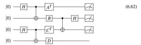
Since the qubit pairs (0, 1) and (2, 3) are each in the  $|\phi^+\rangle$  state, one can apply the ricochet property to move the middle two gates  $(B \text{ and } C^T)$  outward
