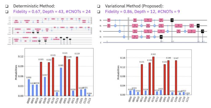
Figure 7.2: Comparison of Deterministic and Variational Methods to prepare the Dicke state  $\left|D_2^4\right>$
