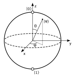
Figure 2.1: Depiction of a qubit  $|\psi\rangle$  on the Bloch sphere
