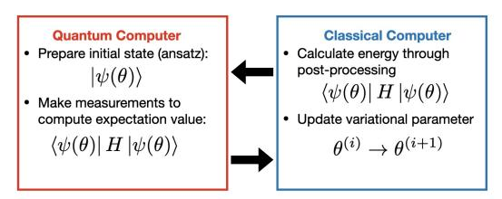
Figure 2.2: Schematic of the Variational Quantum Eigensolver
