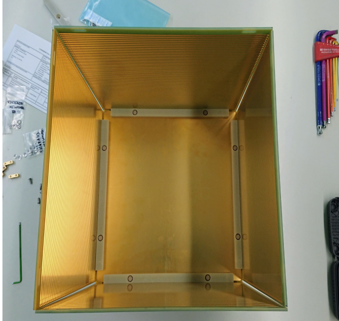
Figure 7.5: SLAC Cube TPC outfitted with a resistor-chain type field shaping device.
