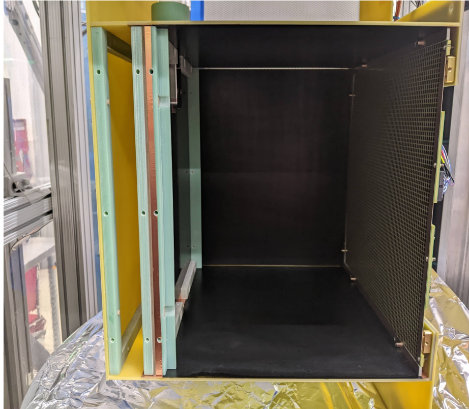
Figure 6.17: The SLAC Single Cube system outside of the cryostat, showing the single-sided TPC with one wall missing. Seen is the cathode (left), a single LArPix tile (right), and a custom carbon-doped sprayed epoxy field cage forming the remaining walls.
