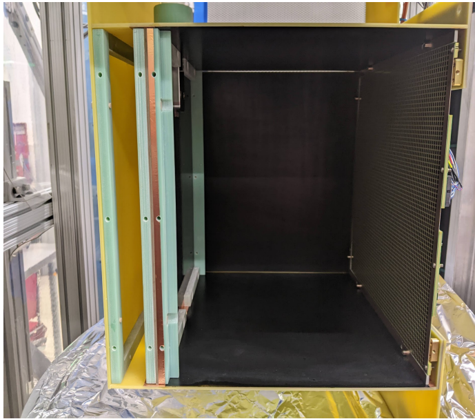
Figure 7.6: SLAC Cube TPC outfitted with a carbon coating type field shaping device.
