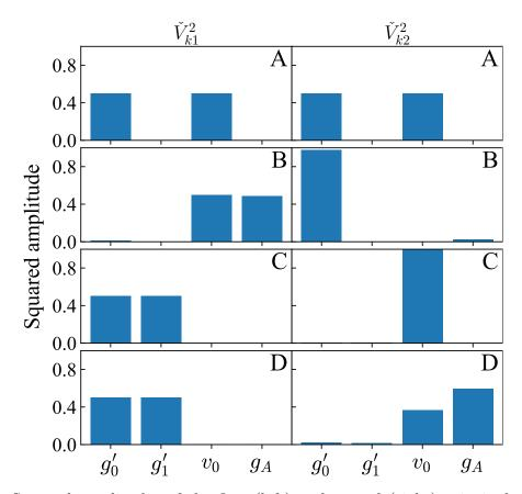
Figure 5.5: Squared amplitudes of the first (left) and second (right) principal components (column vectors of  $\check{V}$ ) that correspond to the first and second largest singular values, for the four fits presented in Table 5.6. They are obtained from Eq. (5.12), the SVD of the normalized Jacobian matrix  $\check{J}$ .
