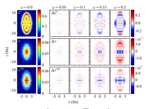
Figure 3.11:  $C^{\tau}$  (top),  $\tau$  (in fm<sup>-5</sup>, middle) and  $\tau^{TF}$  (in fm<sup>-5</sup>, bottom) in the x-z (y = 0) plane, obtained from the CHO model. The leftmost column shows the reference plots at  $\omega = 0$  while the other columns show the rotational dependence relative to the  $\omega = 0$  reference as a function of the rotational frequency  $\omega$  (in units of  $\omega_0$ ).
