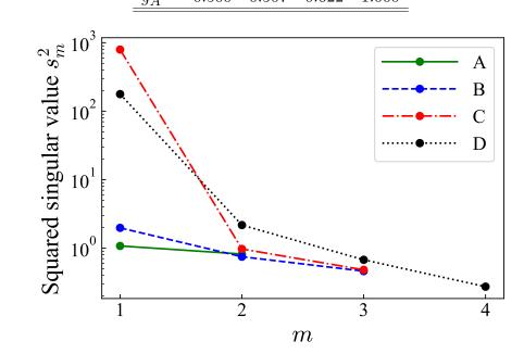
Figure 5.4: Squared singular values (in descending order) obtained from Eq. (5.12), the SVD of the normalized Jacobian matrix  $\check{J}$ , for the four fits presented in Table 5.6.
