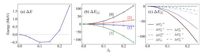
Figure 4.1: The octupole deformation energy  $\Delta E$  of  $^{224}\mathrm{Ra}$  (a), its multipole expansion  $\Delta E_{[L]}$  (b), and the components of the octupole part  $\Delta E_{[3]}$  in isospin and proton-neutron representations (c), as functions of the octupole deformation  $\beta_3$ .
