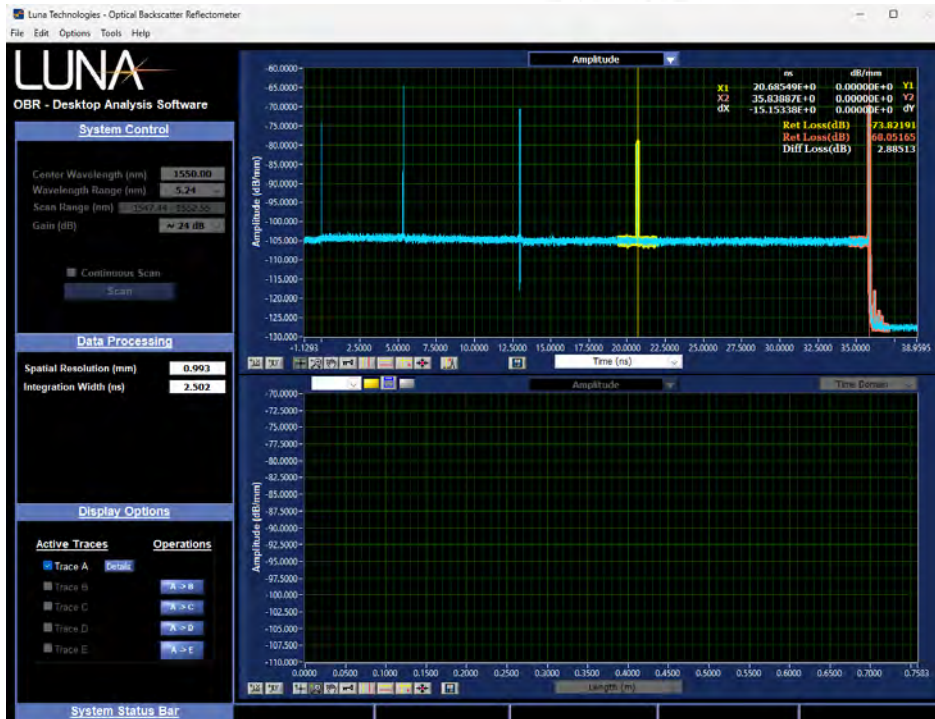
Figure 3.13 Top: An example of what two cable measurements look like with the OBR 4600. The length is determined by multiplying the time by the speed of light, with the difference in time (95 picoseconds) corresponding to a length difference of 19.3 millimeters. Figure is from [23]. BOTTOM: The actual user interface for the OBR. The yellow spike indicates the start of the cable with the orange region being the end. The software automatically finds the time-location of the highest amplitude and calculates the distance between them. Photo courtesy of Pat Harding at LANL.
