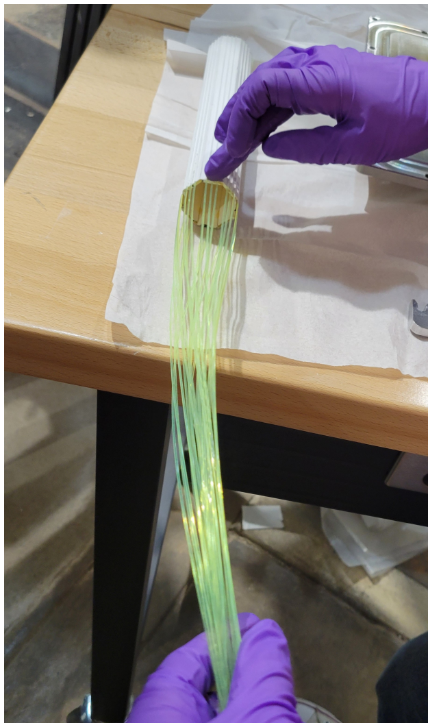
Figure 4.4 Picture of the plastic scintillator, SuNSPOT, with 32 wave-shifting optical fibers glued on the six sides, which is optically coupled to two PMTs to detect the \beta -particles.
