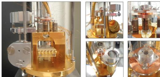
Couple ultrafast **terahertz** pulses to the tip of a scanning tunneling microscope to control electron motion
