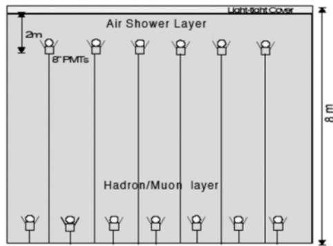
Fig.. 3. Cross sectional schematic of Milagro.
