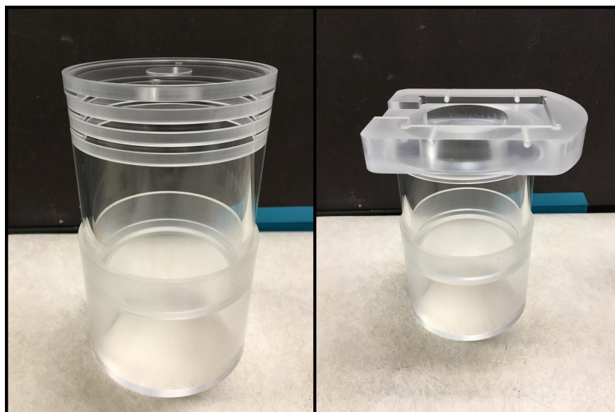
Figure 6.15: custom-designed gamma-source holder for the LLNL HPGe detector.
