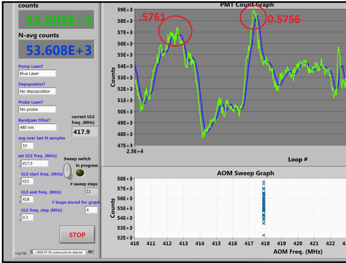
Figure 4.9: A screenshot of the VI I wrote for recording PMT counts for the branching ratio measurements. On the main graph, the raw PMT count is plotted with a user-defined N -sample average. The bottom graph plots the acousto-optical modulator frequency setting. The user can run a laser sweep with a frequency step size of their choosing. The filters installed on the PMT and the lasers being used are specified in the box on the left and the settings are mapped to integers which are saved to a text file along with the PMT counts and AOM settings.
