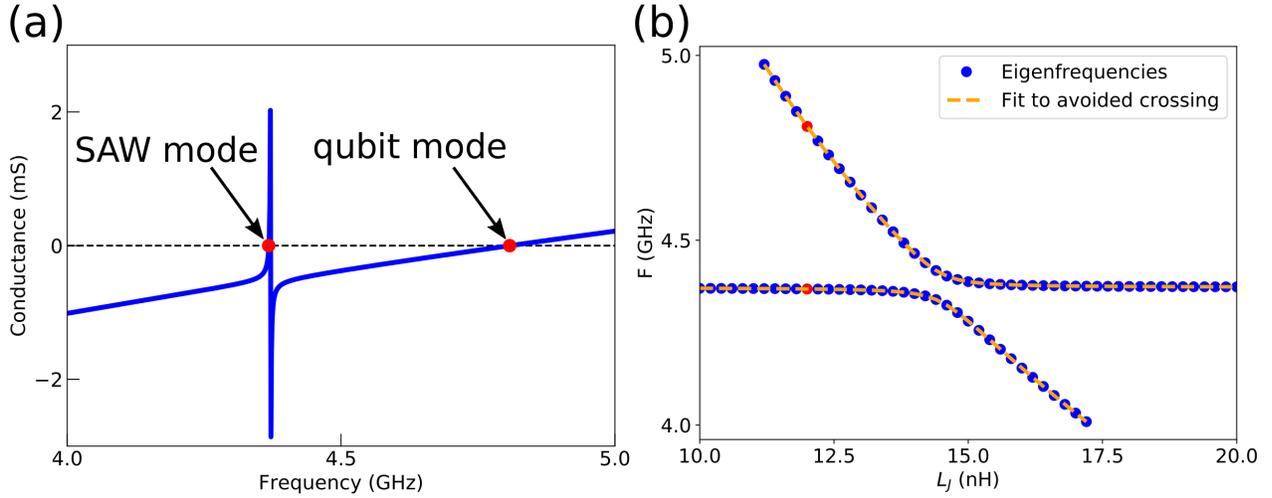
Figure 6.4: (a)  $\text{Im}(Y(f))$  of the linear component of the circuit in Fig. 6.1(d), using element values extracted from FEM/COM modeling and  $L_J = 12$  nH. The zero crossings (red dots) signify a resonance of the circuit. (b) For each value of  $L_J$ , we extract the zero crossings of  $\text{Im}(Y(f))$  (blue dots, red dots correspond to data from panel (a)) and fit to extract the Hamiltonian parameters.
