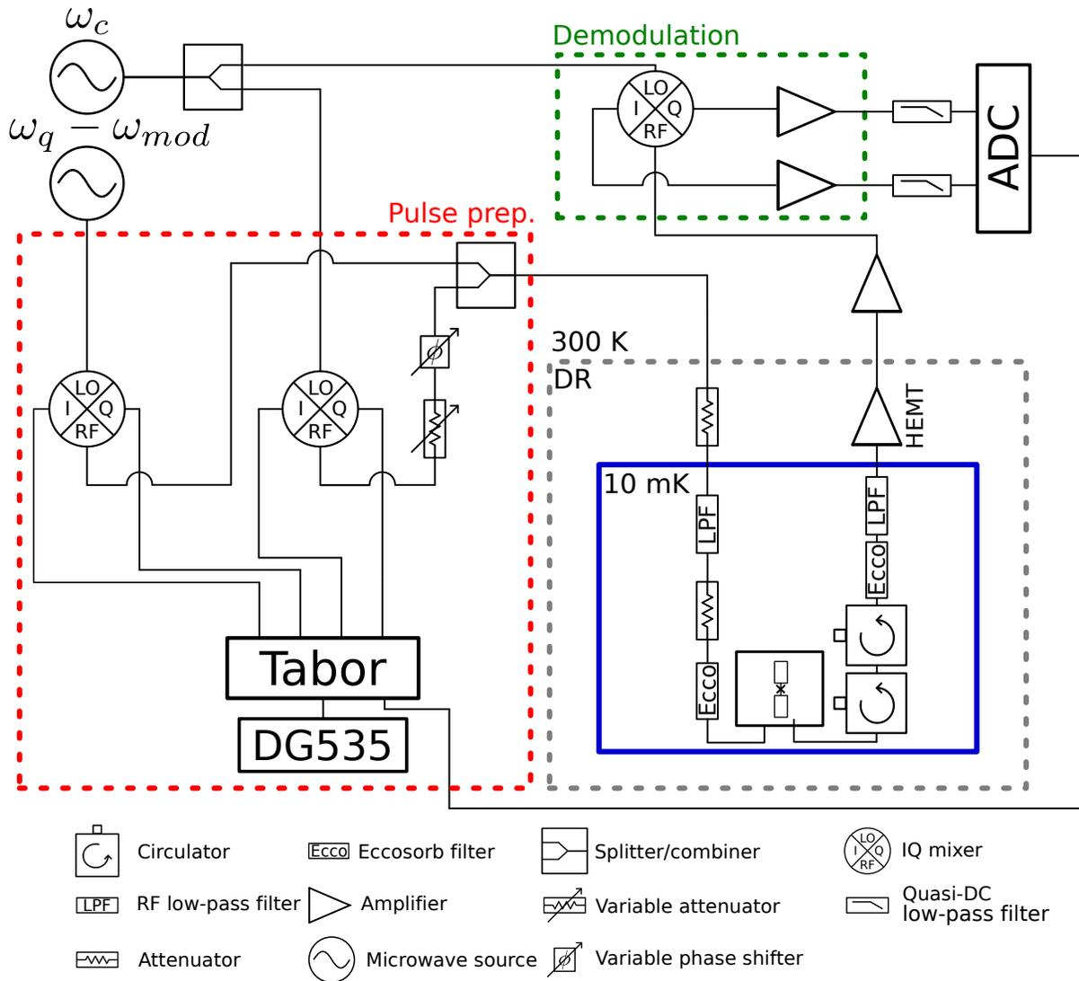
Figure 3.8: A schematic diagram of the most general measurement setup employed when doing time-resolved measurements in this thesis.
