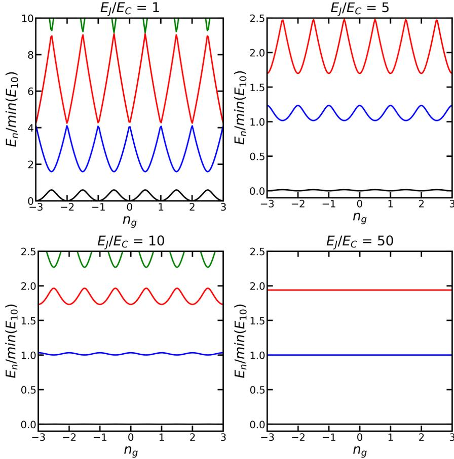
Figure 2.3: Eigenvalues of the Cooper pair box Hamiltonian, as a function of offset charge  $n_g$  for various ratios  $E_J/E_C$ . As the ratio  $E_J/E_C$  goes up, charge dispersion is exponentially suppressed, but anharmonicity is also suppressed. Reproduced from Ref. [34].
