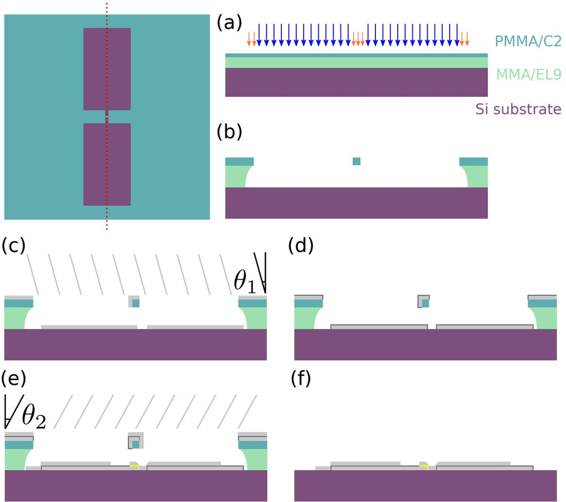
Figure C.1: Process flow of the Dolan bridge junction fabrication process. Top-right: a top down view of the substrate with a resist bridge defined via electron beam lithography. All cross sections (a-f) run along the red dotted line. In panels (e-f), the part of the oxide layer that defines the junction is highlighted in yellow. Note that distances are not to scale.
