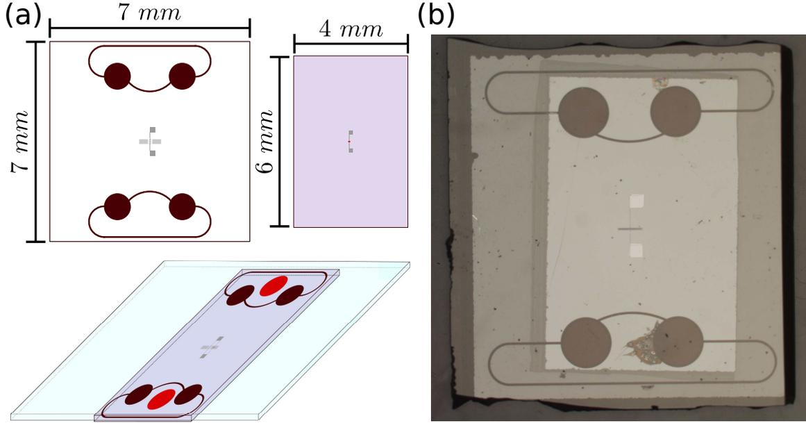
Figure 6.7: (a) Schematics of the devices cut to size, as well as a rendering of the assembled flip-chip stack. The SAW device is made larger than the qubit device for ease of assembly/handling. We use hard baked photoresist (maroon) spacers at the end of the chip to control the spacing between chips, and use soft-baked photoresist (red) to glue the chips together. (b) Image of the flip-chip stack, as seen through the clear LiNbO<sub>3</sub> substrate.
