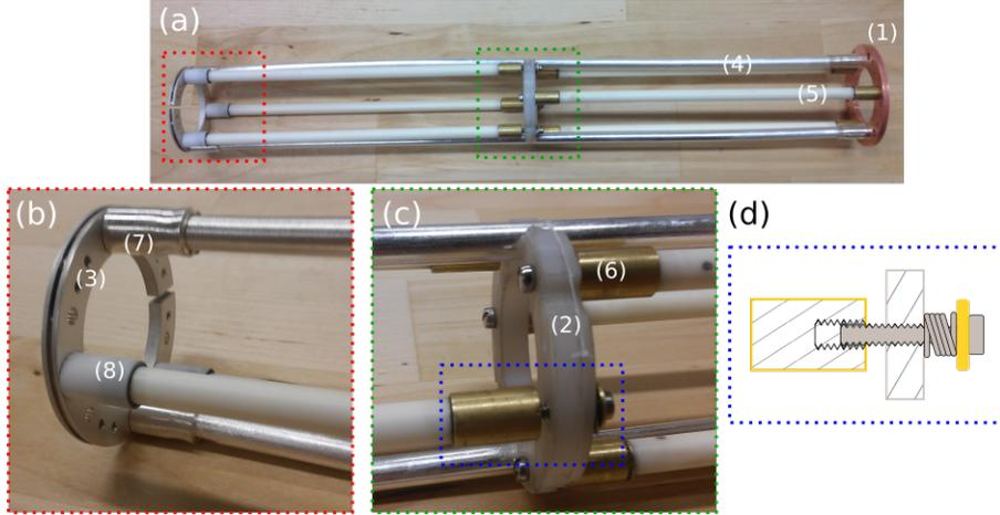
Figure 7.3: (a) Photo of the cold-finger. A copper disk (1) is attached to the MXC plate, and annealed silver rods (4) provide thermalization to the silver sample mounting disk (3). Alumina rods (5) provide structural support. Close up views of (b) the sample mounting disk and (c) the teflon intermediate disk. (d) Mechanism at the intermediate disk for compensating for the discrepancy between the thermal expansion coefficients of alumina and silver upon cooling to cryogenic temperatures.
