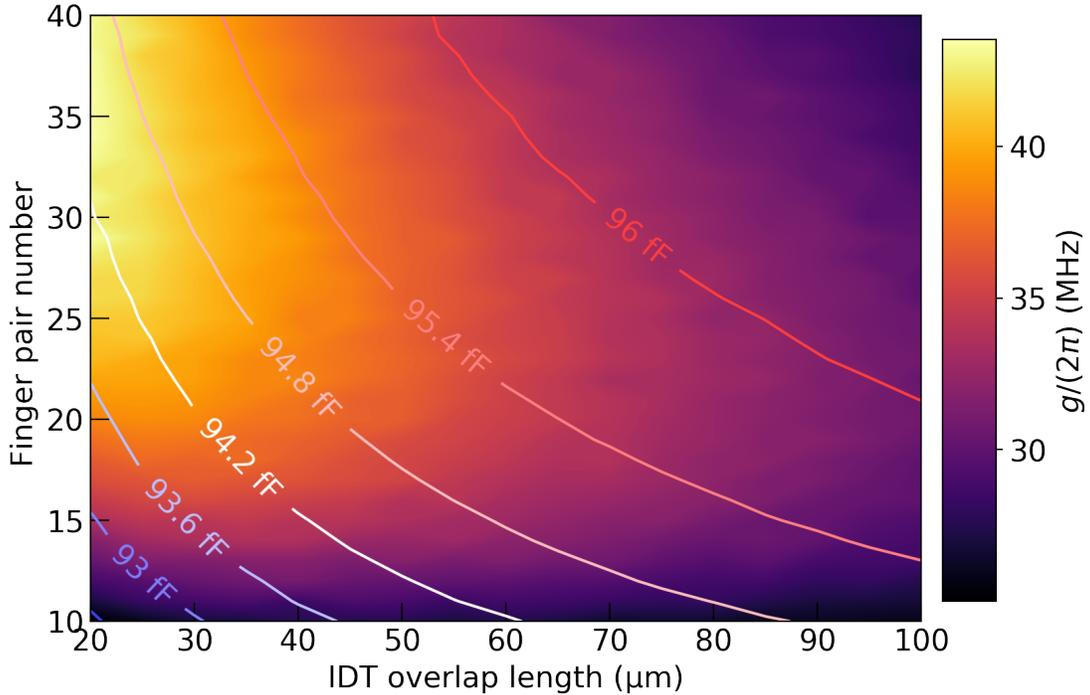
Figure 6.5: Color plot: SAW-qubit coupling  $g_m$  as a function of finger pair number  $N_p$  and IDT overlap length  $w$ . Contours: Transmon mode capacitance  $C_{eff}$  as a function of finger pair number  $N_p$  and IDT overlap length  $w$
