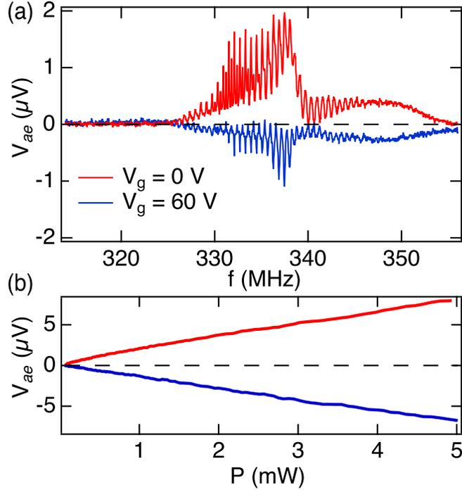
Figure 7.7: (a) Acoustoelectric voltage versus frequency for two gate voltages:  $V_g = 0$  V (hole-doped graphene) and  $V_g = 60$  V (electron doped graphene) at 3.2 K. For these measurements 0 dBm of microwave power was used to excite SAWs. (b) Acoustoelectric voltage as a function of power applied to the SAW circuit, for the same back gate voltages as in panel (a). This data was taken at a fixed frequency  $f = 337.45$  MHz corresponding to the maximum in the response of the SAW transducer.
