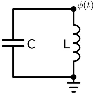
Figure 2.1: A parallel LC circuit. We have defined two nodes: one at ground, and one at node flux relative to ground  $\phi(t)$
