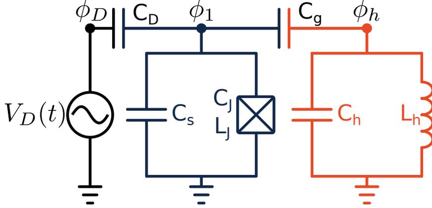
Figure 2.5: A circuit schematic of the circuit quantum electrodynamics (cQED) protocol. A qubit (blue) is coupled to a microwave frequency electromagnetic cavity, modeled as an LC oscillator (orange). We apply microwave qubit control and readout pulses through an external drive (modeled as a voltage source in black.) Here, we take the qubit to be a transmon qubit, and the coupling to the cavity/drive to be capacitive.
