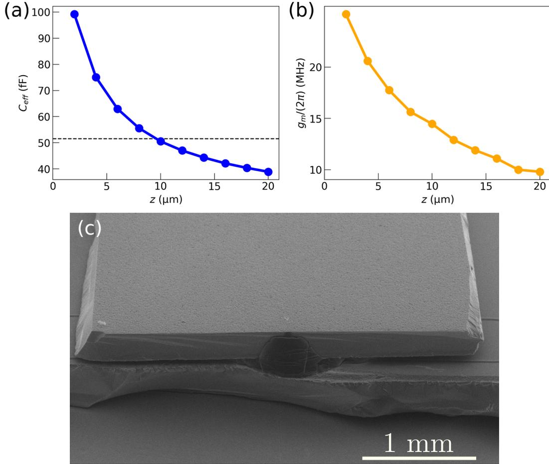
Figure 6.10: (a) Transmon mode capacitance  $C_{eff}$  and (b) acoustic coupling  $g_m$  as a function of height, using the all other parameters from the model outlined in Table 6.2. Empirically determined mode capacitance marked with a dashed black line. (c) SEM picture of the the flip-chip stack from the edge, indicating that the spacing of this chip-stack limited by the glue rather than the hard baked spacers.
