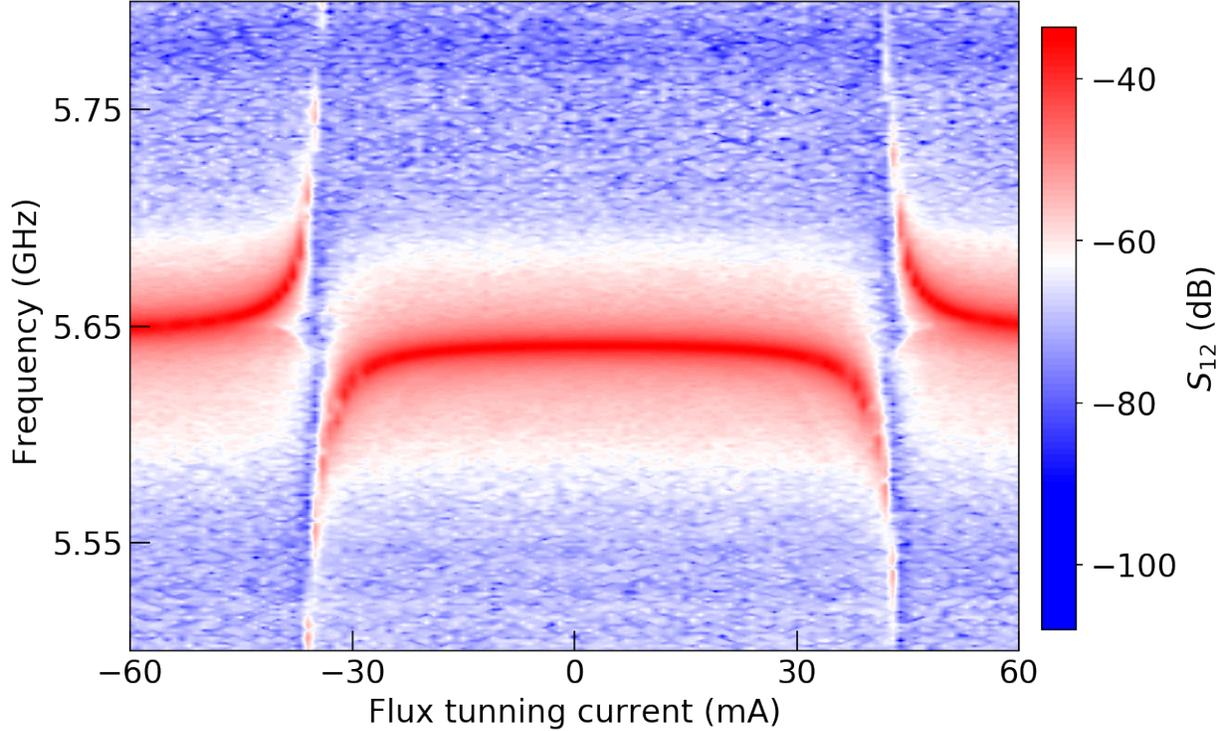
Figure 6.8: Transmission  $S_{12}$  through the 3D electromagnetic cavity with a qubit + ST-X quartz device loaded in, as a function of both frequency and flux tuning current.
