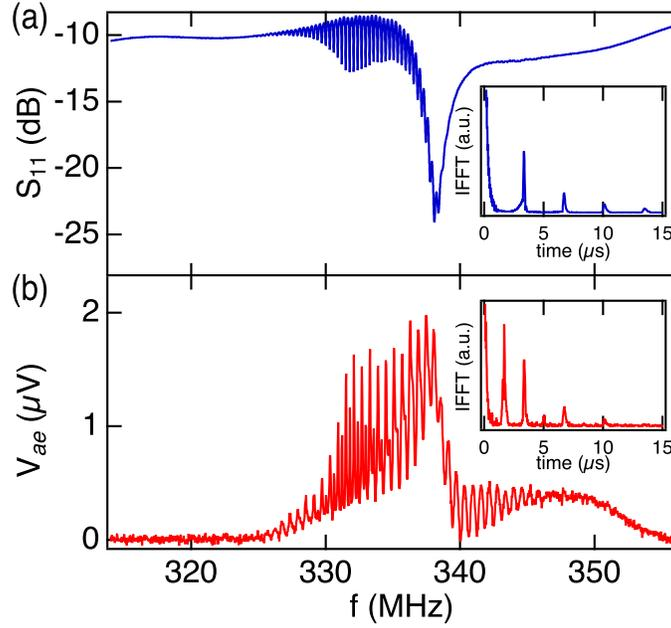
Figure 7.6: (a) Frequency dependence of the reflection coefficient ( $S_{11}$ ) of the SAW delay line. Inset: inverse fast Fourier transform (IFFT) of  $S_{11}$  data. (b) Measured acoustoelectric voltage in the graphene sample as a function of frequency. This measurement was conducted at 3.2 K with the sample back gate grounded. To excite the SAW, 0 dBm of microwave power was applied at the top of the cryostat. Inset: inverse Fourier transform of the acoustoelectric signal.
