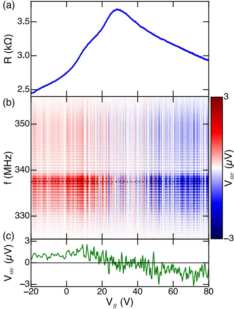
Figure 7.8: (a) Low-frequency two-point resistance of the graphene sample as a function of back gate voltage. (b) Acoustoelectric voltage signal (taken with 0 dBm of SAW power), plotted as a function of both back gate voltage and SAW frequency. At gate voltages where the graphene is heavily electron (hole) doped,  $V_{ae}$  is consistently negative (positive). (c) Constant frequency linecut of  $V_{ae}$  at  $f = 337.45$  MHz, indicated by the dashed line in panel (b).
