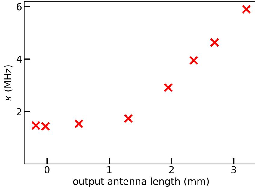
Figure 3.2: Measured decay rate  $\kappa$  of a 3D microwave cavity as a function of the output antenna length with the input antenna length fixed. The length is referenced relative to the inner surface of the microwave cavity (and thus may be negative if the pin is recessed from the cavity wall.) These measurements were taken in a polished copper cavity at  $T \approx 300$  K.
