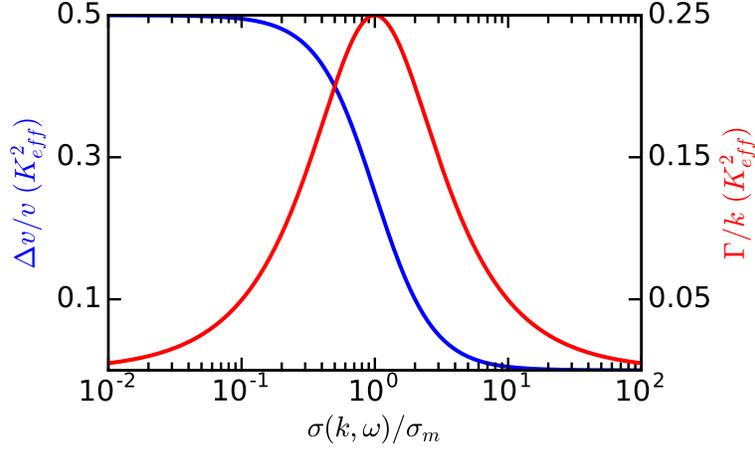
Figure 7.2: Relative SAW velocity shift  $\Delta v/v$  (blue, left axis) and attenuation per unit length normalized by the SAW wave vector  $\Gamma/k$  (red, right axis) as a function of normalized 2DES conductivity  $\sigma(k, \omega)/\sigma_m$ . Both are given in units of the effective piezoelectric coupling constant  $K_{eff}^2$ .
