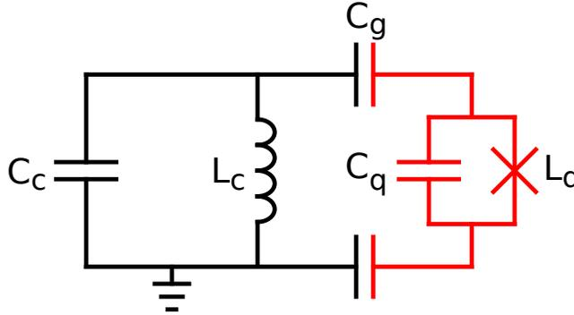
Figure 4.6: Circuit model for a 3D transmon circuit (red/gray) coupled to a linear cavity (black) used to estimate the change in the vacuum Rabi splitting  $\Delta g_{01}$  in the presence of superfluid helium.
