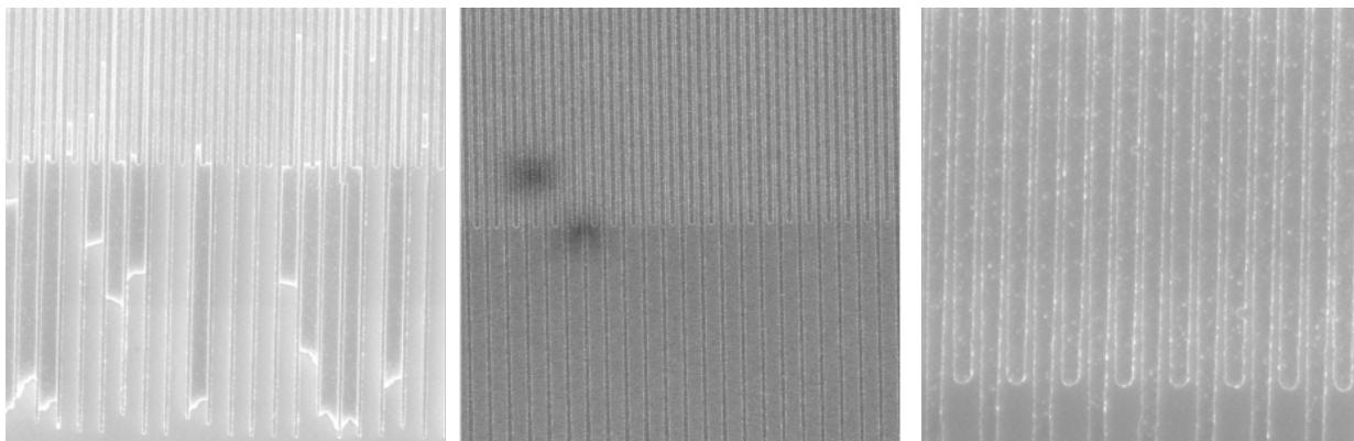
Figure C.3: Left: underdosed SAW IDT. Generally, when the IDTs are underdosed, lift-off is difficult. Center: optimized dose. Lift-off is easy, and  $a \approx b$ . Right: overdosed IDT. Clearly in this case,  $a \gg b$ , however even though the space between the IDT fingers is very small, lift-off generally goes well. Eventually, at too high a dose, lift off will get spotty right before the IDTs simply short together.
