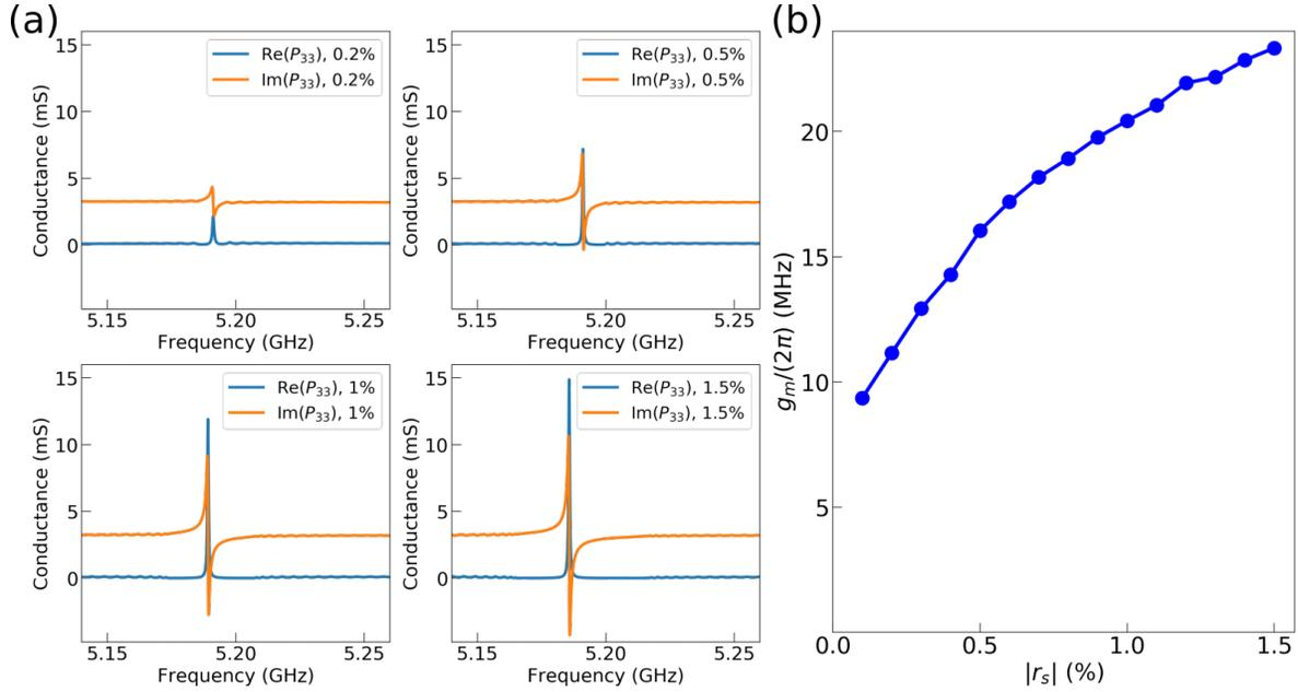
Figure 6.11: (a) Real (blue) and imaginary (orange) parts of the acoustic admittance  $Y = P_{33}$ , calculated using various values of the per-grating reflectivity. As the reflectivity decreases, the electrical response of the resonator becomes weaker. (b)  $g_m$  calculated at various values of  $|r_s|$  using all other values defined in Table 6.2.
