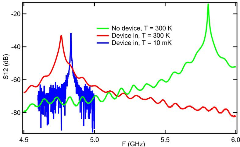
Figure 6.13: Transmission of a 3D cavity at room temperature with no device (green), at room temperature with a LiNbO<sub>3</sub>/silicon flip-chip stack (red), and at  $\sim 10$  mK with a LiNbO<sub>3</sub>/silicon flip-chip stack (blue). Note that the absolute magnitude of the low temperature also encapsulates the experimental attenuation/amplification, and should therefore not be directly compared to the magnitude of the other data.
