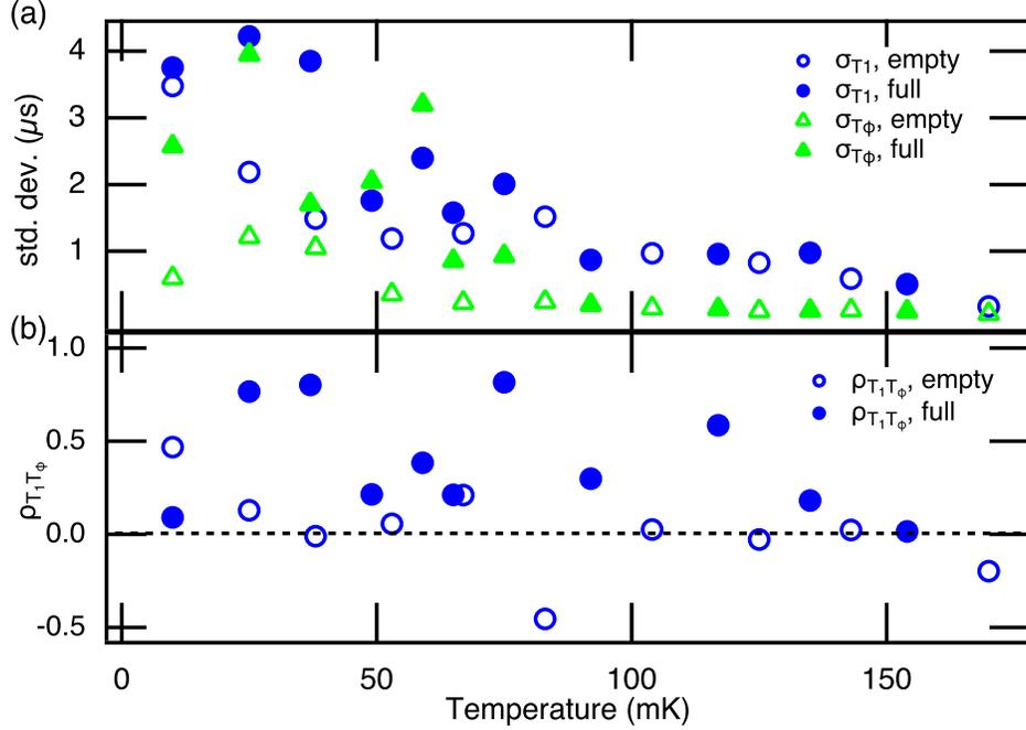
Figure 4.9: (a) Standard deviation of the measured datasets of  $T_1$  and  $T_\phi$  for both empty and full cavities. (b) Normalized covariance of the sets of measured  $T_1$  and  $T_\phi$ .
