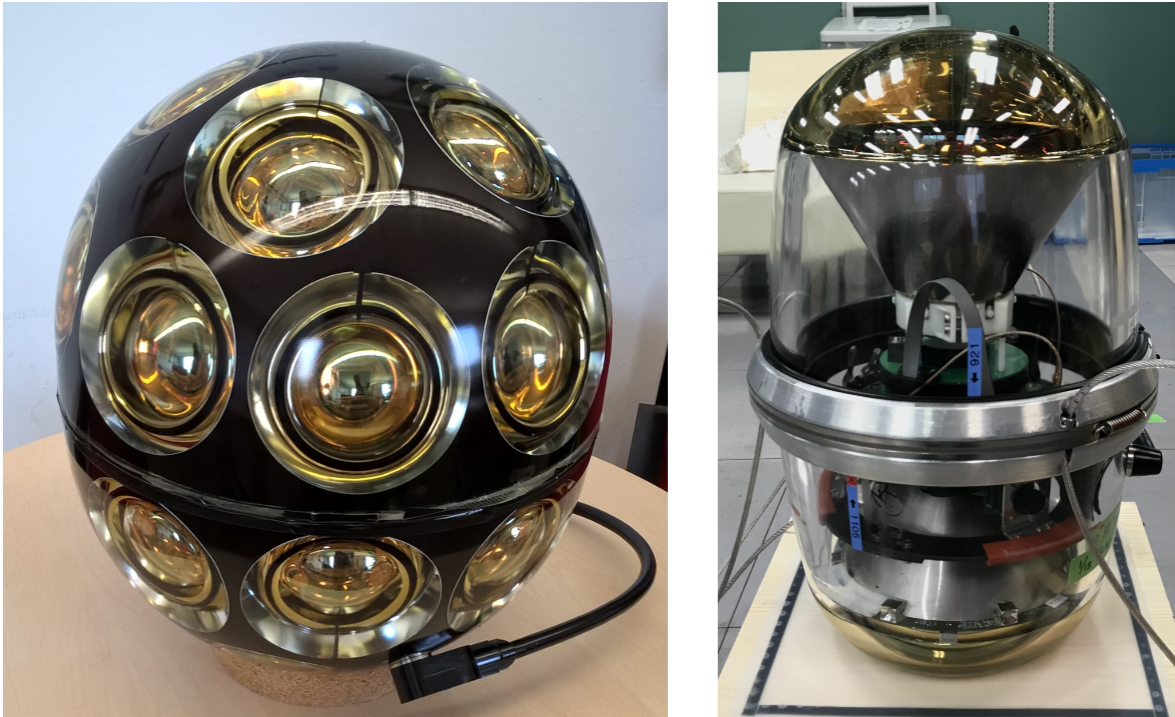
Figure 3.16: Showing an mDOM (left) and a D-Egg (right), the two main optical modules to be used in the IceCube Upgrade [29].
