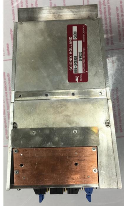
Figure 3.1: **HiRA10 Telescope** Left: HiRA10 mechanical drawing. Right HiRA10 Telescope picture. Discoloration to the can comes from the basic nature of the cleaning detergent used to clean the parts. (If you use a basic cleaner (ph >9), aluminum parts may acquire dark brown and black splotchy marks. For aluminum parts a neutral cleaner with ph 7 is needed.)
