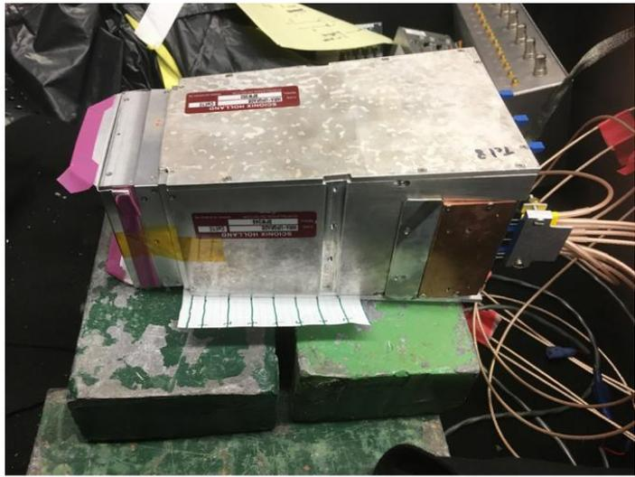
Figure 2.16: **Gamma Test Setup** Left: Gamma source collimator setup. Right: HiRA10 in gamma testing setup. The telescope is placed on top of the collimator. The note card beneath the telescope has been marked such that then one of the delineation on the card is lined up with the edge of gap in the collimator a 1 cm wide section of the CsI(Tl) crystals is illuminated with the gamma source.
