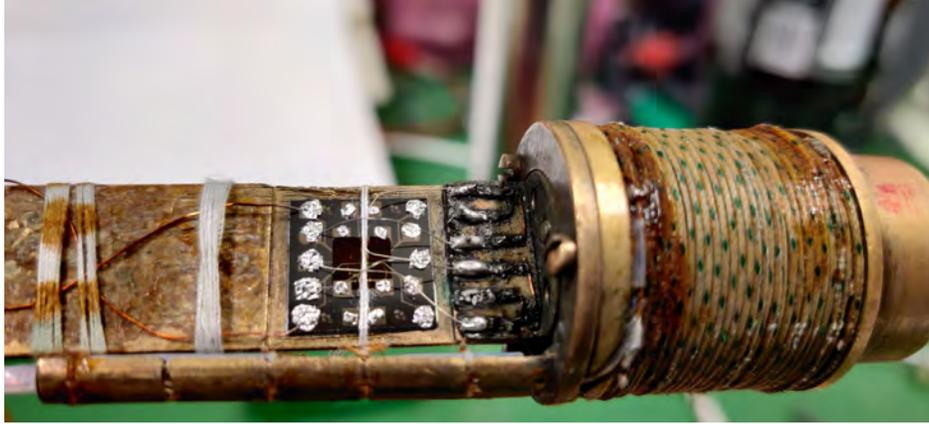
Figure 4.7: *Sample mounted on QDI*: Electrical connections using Indium for sample mounted on QDI.
