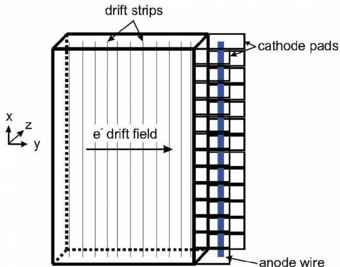
Figure 3.3: A schematic of a CRDC detector used in the S800 focal plane. The beam axis  $z$ , dispersive axis  $x$ , and non-dispersive axis  $y$  are shown. The image is from Ref. [70].
