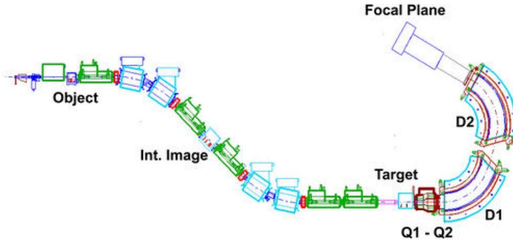
Figure 3.1: A schematic of the S800 spectrograph. The figure is from Ref. [70].
