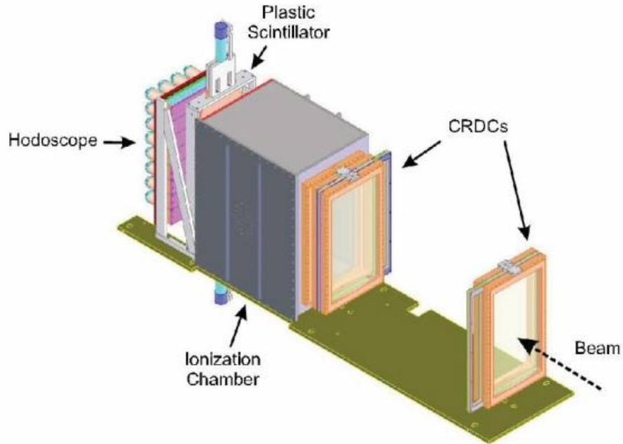
Figure 3.2: The S800 focal plane. The cathode readout drift chambers (CRDC's), plastic scintillator (E1 scintillator), ionization chamber, and IsoTagger hodoscope are depicted. The image is from Ref. [70].
