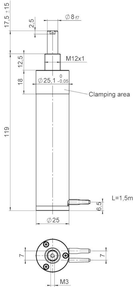
Figure 3.16: A schematic of a motor used to drive a tube and foil in the TRIPLEX device. The image is from Ref. [85].
