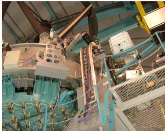
*Spartan Camera mounted on the Nasmyth focus of the SOAR Telescope. Spartan is the white box to the right of center, while the bottom of SOAR's primary mirror cell and the ring at the top of the telescope that holds the secondary mirror fill the*
