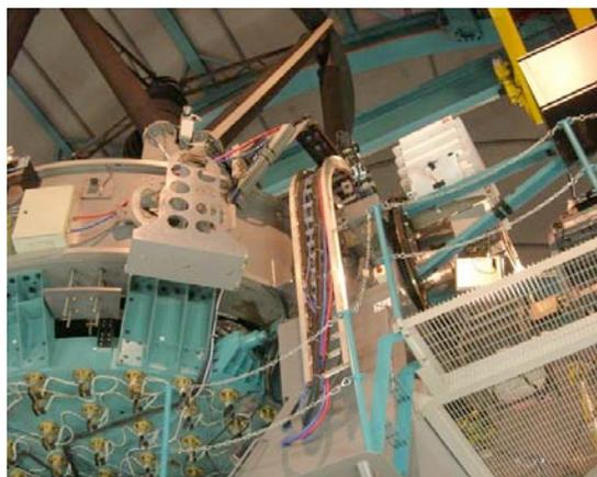
*Spartan Camera mounted on the Nasmyth focus of the SOAR Telescope. Spartan is the white box to the right of center, while the bottom of SOAR's primary mirror cell and the ring at the top of the telescope that holds the secondary mirror fill the*
