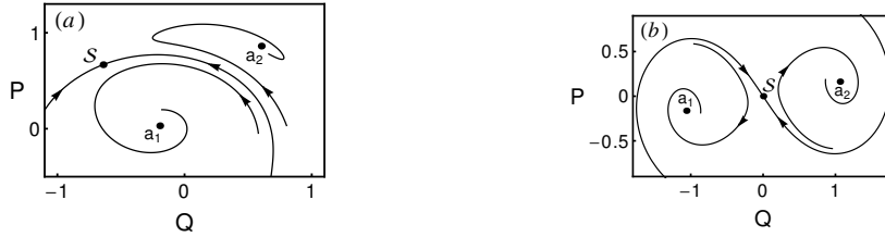
Fig. 7.5 The phase portraits of the classical additively (a) and parametrically (b) modulated oscillators in the rotating frame. The attractors a_{1,2} correspond to the stable states of forced vibrations in the lab frame. Their positions (Q_a, P_a) give the scaled vibration amplitudes A_{\text{osc}} = (Q_a^2 + P_a^2)^{1/2} in Fig. 7.1. The separatrix that goes through the saddle point S is the boundary of the basins of attraction to different attractors. The phase portrait in (b) has inversion symmetry. The parameters in (a) are \beta = 1/27 , \kappa = 0.15 ; in (b) \mu = 0.2 , \kappa = 0.3 .
