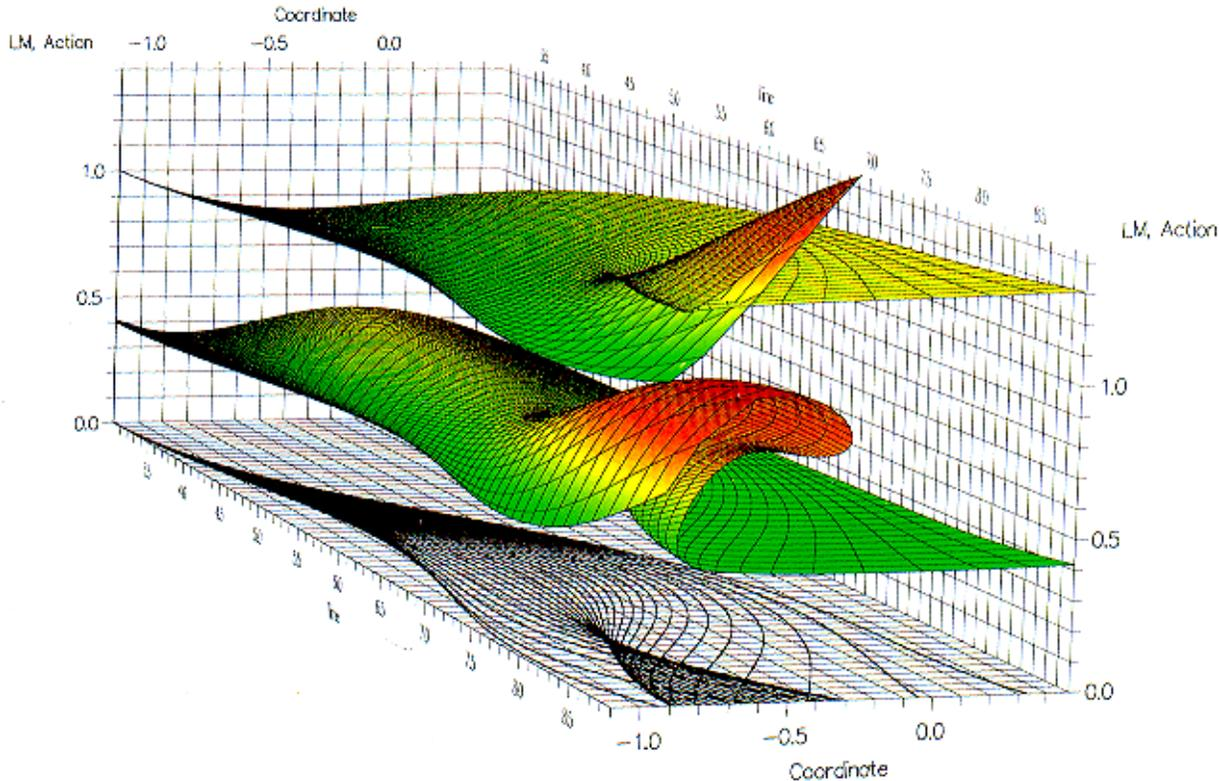
Fig. 1. From top to bottom: action surface, Lagrangian manifold (LM) and extreme paths calculated for the system (2) using Eq. (6) with initial conditions (9). Parameters for the system were:  $A = 0.264$ ,  $\omega = 1.2$ . To clarify interrelations between singularities in the optimal paths pattern, action surface, and LM surface, they are shown in one figure: the action surface has been shifted up by one unit, and the LM scaled by a factor 1/2 and shifted up by 0.4.
