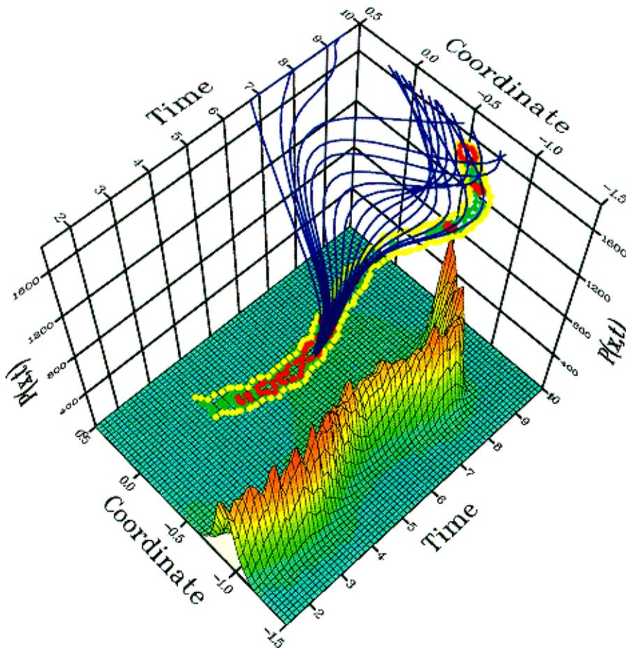
Fig. 2. Distribution of fluctuational paths which terminate inside the rectangle  $-0.7 \leq q_f \leq -0.65$ ,  $9.0 \leq t_f \leq 9.2$  for the system (2) with  $A = 0.264$ ,  $\omega = 1.2$ . The maxima of the distribution represent the optimal paths. The theoretical extreme paths and the contour plot of the distribution are shown at the top.
