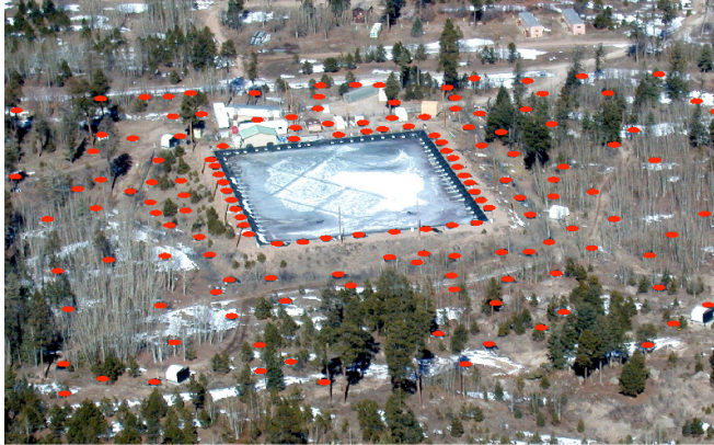
Figure 2: Aerial view of the Milagro detector. The central pond is visible and the red dots indicate the locations of the outriggers.
