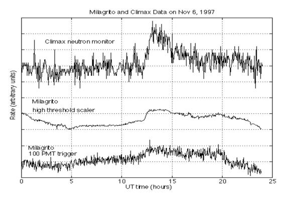
Figure 2. Milagrito registered a rate increase coincident with that of Climax during the GLE of Nov. 6, 1997. The yaxis units have been scaled and shifted for each plot to make comparison easier. (Climax data courtesy of C. Lopate, Univ. of Chicago)
