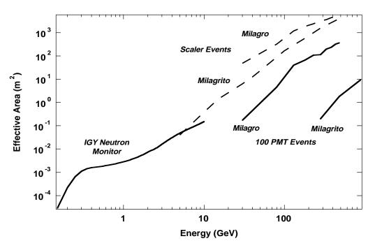
**Figure 1.** Preliminary, lower-limit effective area curves for Milagro and Milagrito, with a sea-level IGY neutron monitor for comparison. (The Milagro shower trigger is no longer set at 100 PMTs, but Milagrito shower data was recorded with a 100 PMT threshold.)
