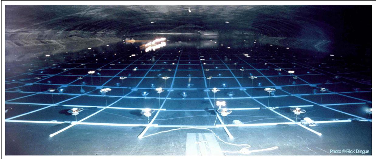
**FIGURE 1.** This photograph shows the Milagro reservoir (80 m x 60 m) from under the light tight cover. Clearly visible are the photo tubes arranged on a 3 m grid. The upper layer of phototubes is under 1.5 m of water, while the second layer is under 7 m of water.
