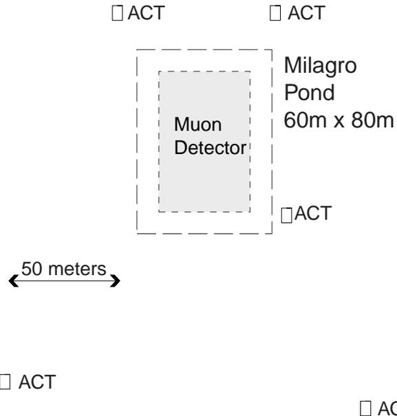
Figure 3: Placement of WACT telescopes relative to Milagro.
