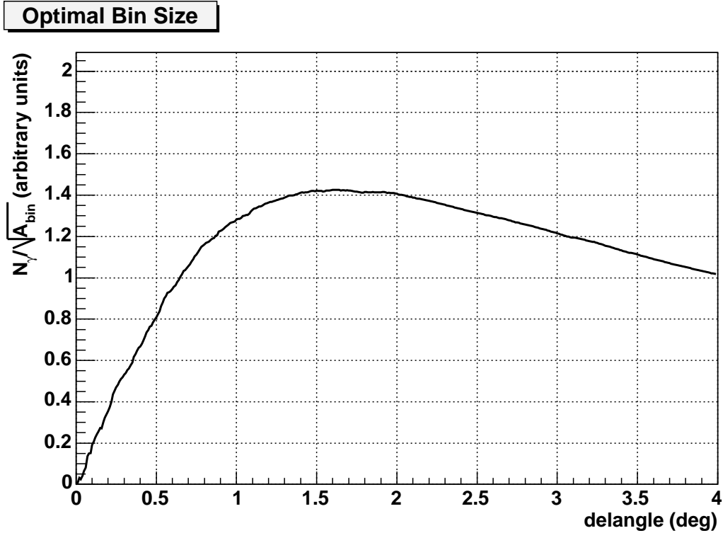
Figure 2.19: Determination of the optimal bin size. From simulations, the number of gamma rays contained within the bin is determined as a function of bin size. The value of the delangle cut that optimizes the ratio of the number of gamma rays to the square root of the area of the bin determines the optimal bin size.
