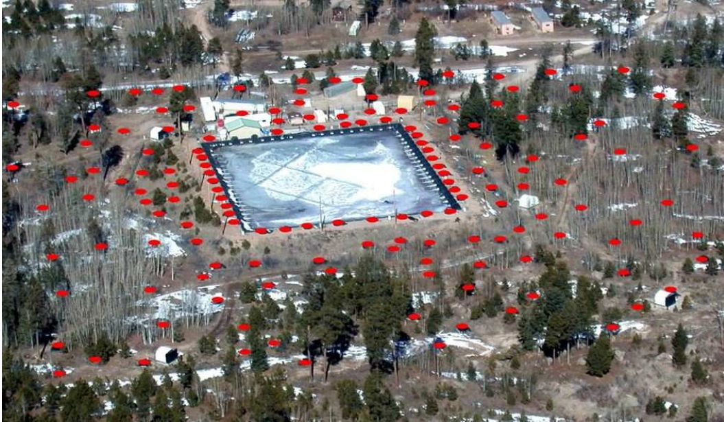
Figure 2.2: Aerial view of the Milagro detector. The rectangular area in the center is the pond. The red disks show the location of the outrigger tanks.
